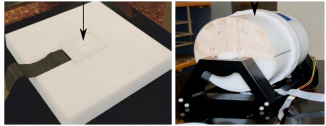
FIG. 2. The slab phantom (left side) and the cylindrical rotating phantom (right side). The arrows show the direction of the beam.
