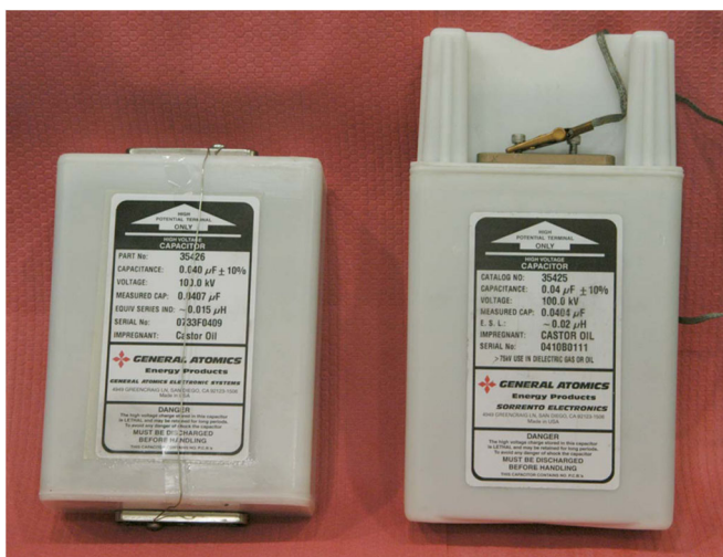
FIG. 3. Comparison of the double-ended 40-nF capacitors used in LTD-III with the single-ended 40-nF capacitors used in previous experiments.
