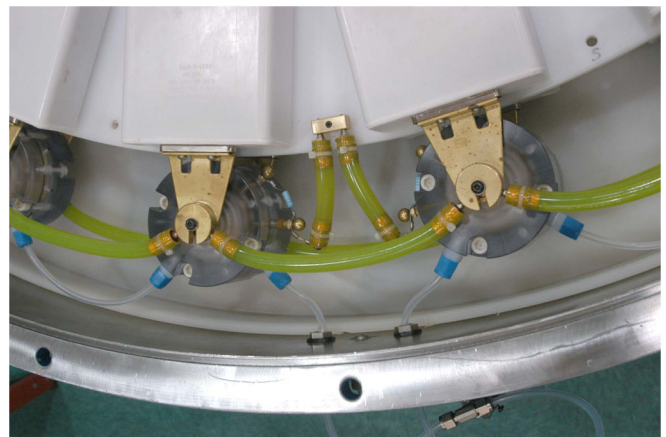
FIG. 7. Details of LTD-III connections with 58-nF capacitors, and all liquid charge and trigger resistors.
