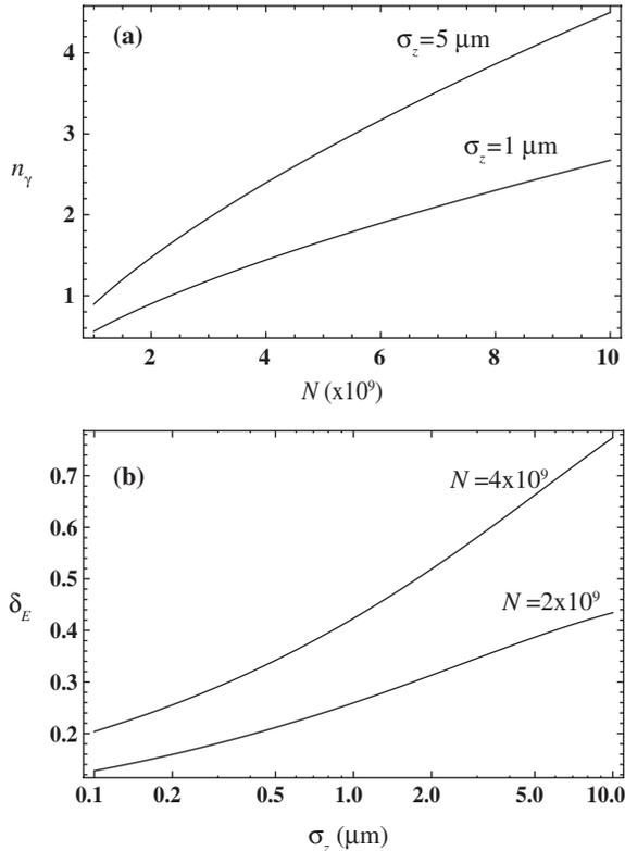
FIG. 4. (a) Beamstrahlung photons emitted per electron  $n_\gamma$  versus  $N$  for bunch lengths  $\sigma_z = 1 \mu\text{m}$  and  $5 \mu\text{m}$ . (b) Beamstrahlung induced energy spread  $\delta_E$  versus bunch length  $\sigma_z$  for  $N = 2 \times 10^9$  and  $N = 4 \times 10^9$ .
