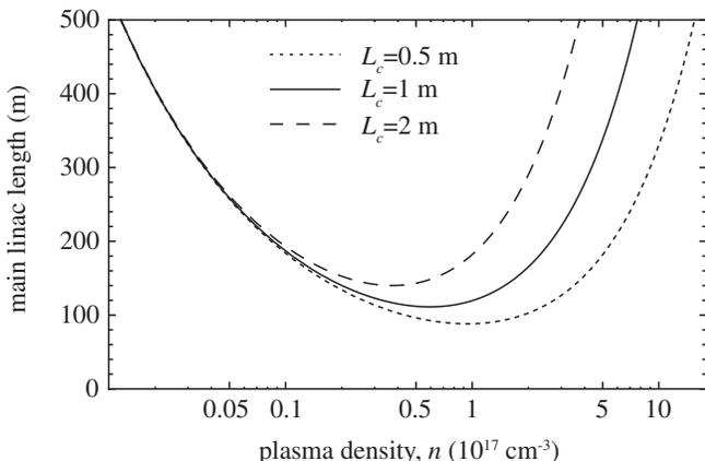
FIG. 3. Main single-linac length versus plasma density  $n$  for several laser in-coupling distances  $L_c$ , for  $E_b = 0.5$  TeV and  $a_0 = 1.5$ .
