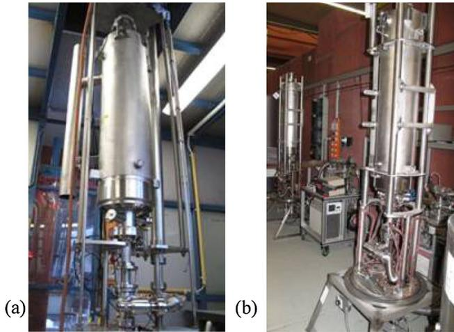
FIG. 2. (Color) (a) Cavity equipped with helium tank and all accessories installed to the vertical test insert. (b) Cavity dressed with helium tank installed to 120°C baking apparatus before vertical rf measurement.
