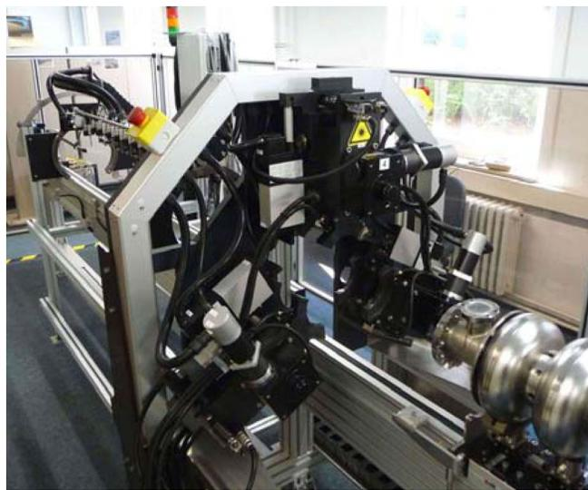
FIG. 17. (Color) The picture shows the tuning frame with the baseplate and the three vice units. On the cable channel the emergency switch is assembled.
