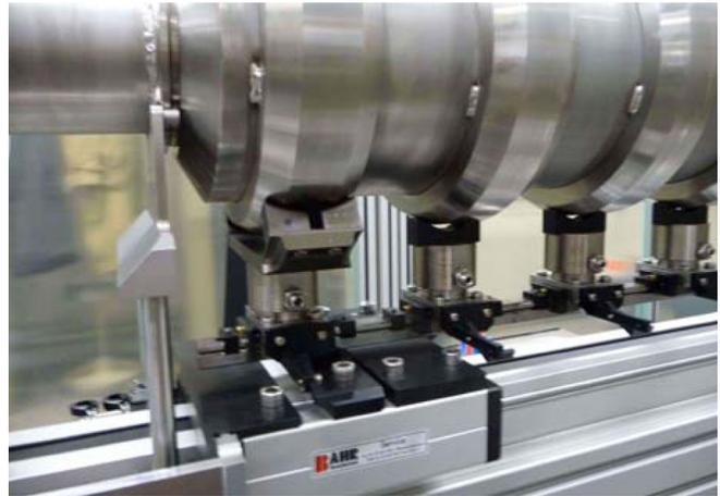
FIG. 19. (Color) Lift units and CT supports with the lift units at the left, contacting the reference plane. A dummy cavity is used to calibrate the eccentricity measurement device.
