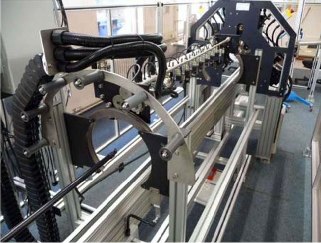
FIG. 20. (Color) Eccentricity measurement device, showing the rotatable arm with the distance generators.
