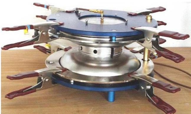
FIG. 8. (Color) Simple rf-measurement device with clamped dumbbell.
