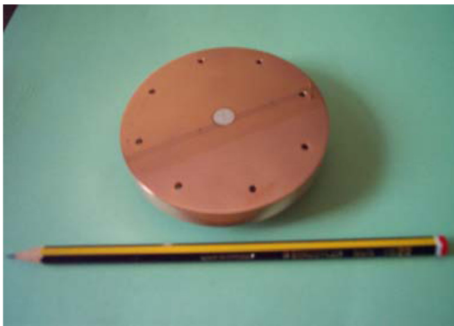
FIG. 2. (Color) Picture of the Cu backflange. At the center is clearly visible the Mg film.
