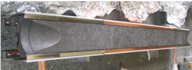
FIG. 2. (Color) A collimator jaw of the same type as installed in the SPS. The figure is taken from [31].
