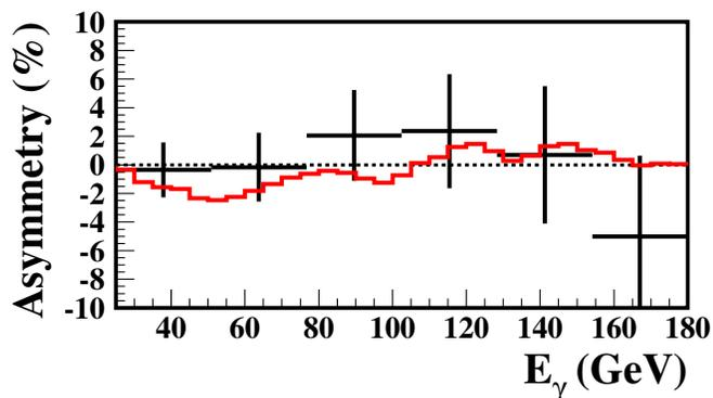
FIG. 27. (Color) Asymmetry of the  $e^+e^-$  pair production in the aligned diamond crystal as a function of the photon energy  $E_\gamma$  which is measured to determine the  $P_1$  component of the photon polarization in the SOS-aligned Si crystal by 178 GeV electrons. The black crosses are the measurements and the red histogram represents the Monte Carlo prediction.
