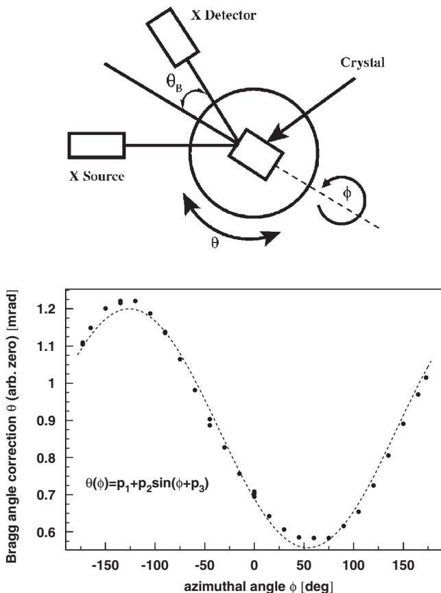
FIG. 11. Schematic setup (top) and measurements of the Bragg peak adjustment angle  $\theta$  as a function of the azimuthal rotation angle  $\phi$  (bottom) for the annular stage alignment of the quarter wave plate crystal with x rays.
