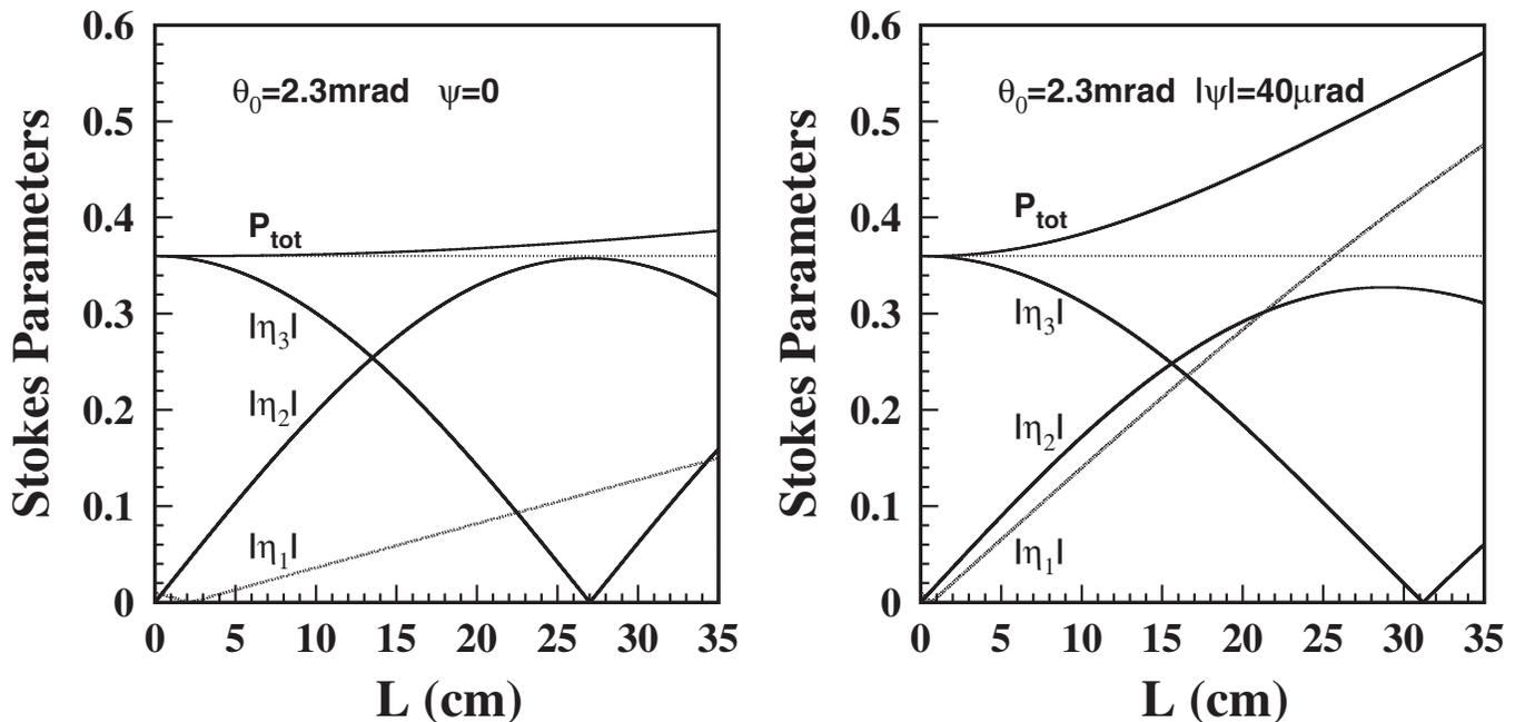
FIG. 8. (Color) Absolute values of the Stokes parameters and the total degree of polarization for a Si crystal as a function of its thickness  $L$ , for  $E_\gamma = 100$  GeV linearly polarized photons. The left-hand figure and the right-hand figure are calculated using initial values for the Stokes parameters described in the text. For these conditions, the crystal also acts as polarizer generating a  $\eta_1$  component.
