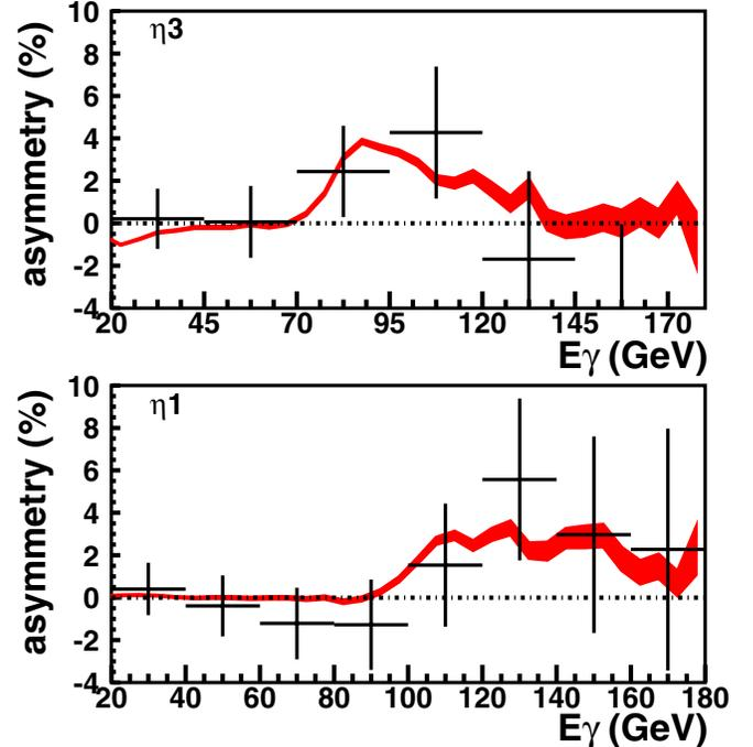
FIG. 22. (Color) Asymmetry measured with the Ge analyzer (top) and the pair spectrometer (bottom). The data sample with a fully reconstructed single  $e^+e^-$  pair is 10 times smaller than the total data sample with at least one pair passing all the data quality cuts and with a 2MIPs cut (see Sec. IVA) in S11.
