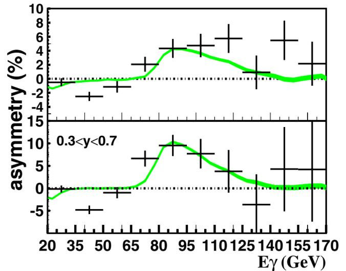
FIG. 16. (Color) Asymmetry to determine the  $\eta_3$  component of the CB photon polarization with the Ge analyzer. Measurements without (top) and with (bottom) the quasisymmetrical pair selection at roll angles  $0 + \pi$  are compared to those at roll angles  $\pi/2 + 3\pi/2$ .
