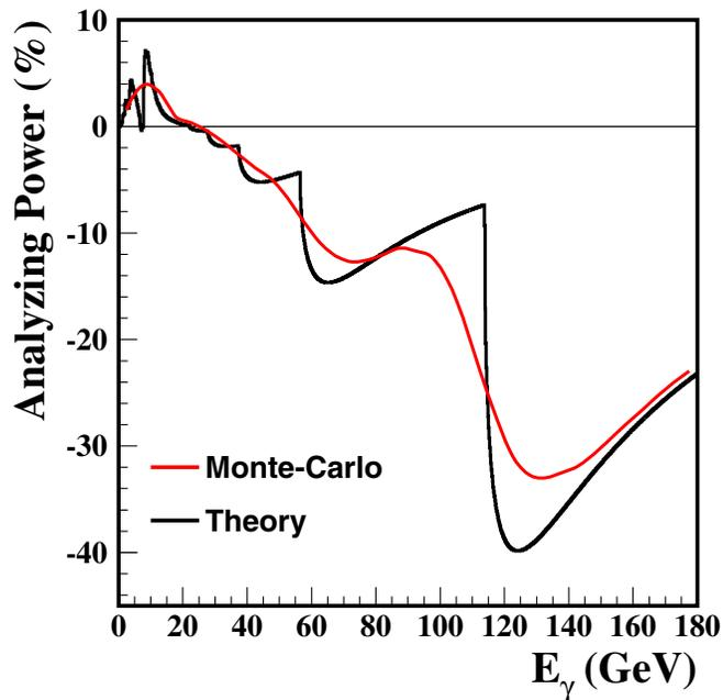
FIG. 26. (Color) Analyzing power  $R$  with the aligned diamond crystal as a function of the photon energy  $E_\gamma$  (black curve) for an ideal photon beam without angular divergence and (red curve) for the Monte Carlo simulation of photons with the beam conditions in the actual experiment.
