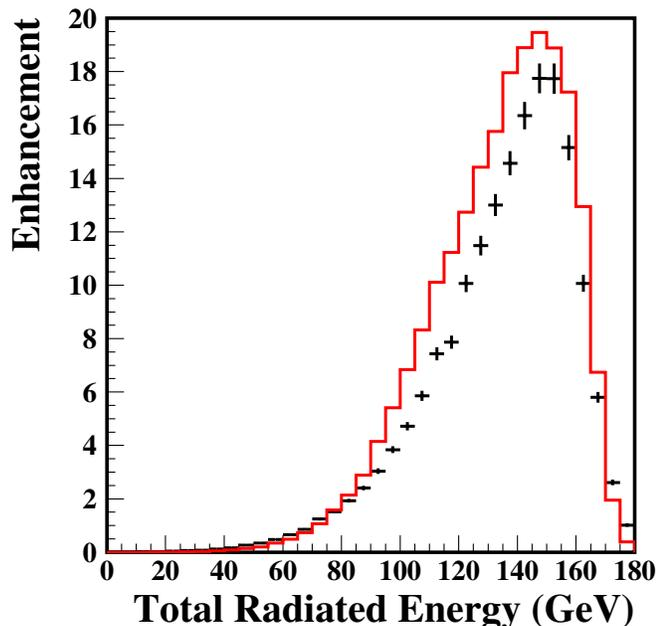
FIG. 24. (Color) Enhancement of the intensity with respect to the Bethe-Heitler (ICB) prediction for randomly oriented polycrystalline Si as a function of the total radiated energy  $E_{\text{tot}}$  in the SOS-aligned Si crystal by 178 GeV electrons. The black crosses are the measurements and the red histogram represents the Monte Carlo prediction.
