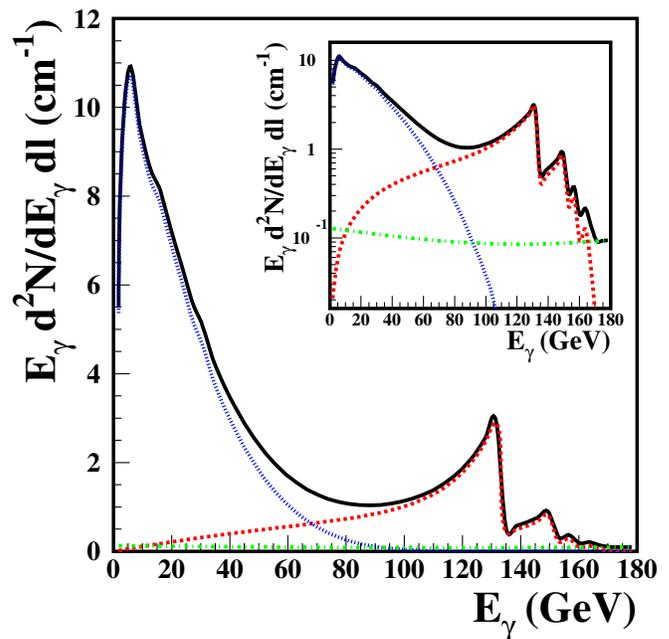
FIG. 3. (Color) Photon power yield,  $E_\gamma d^2N/dE_\gamma dl$ , per unit of thickness for a thin silicon crystal in the SOS orientation. The solid curve represents the total of the contributions from ICB (green dash-dotted), PC (blue dotted), and SOS (red dashed) radiation. The inset is a logarithmic representation and shows the flat incoherent contribution and the enhancement with a factor of about 20 for SOS radiation at 129 GeV.
