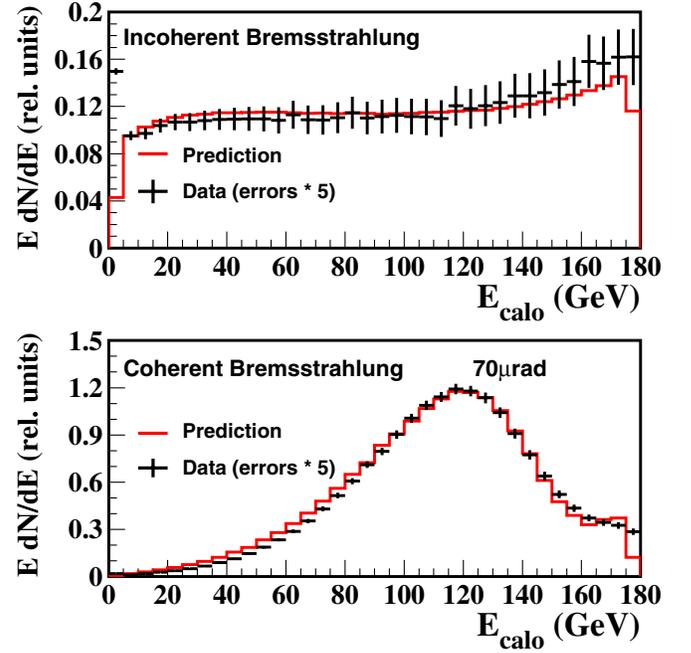
FIG. 13. (Color) Power spectrum for incoherent (top) and for coherent bremsstrahlung (bottom) as a function of the total energy  $E_{\text{calo}}$  detected in the calorimeter. Vertical axis: Power (relative units). The statistical errors on the data are enhanced by a factor of 5 to increase visibility.
