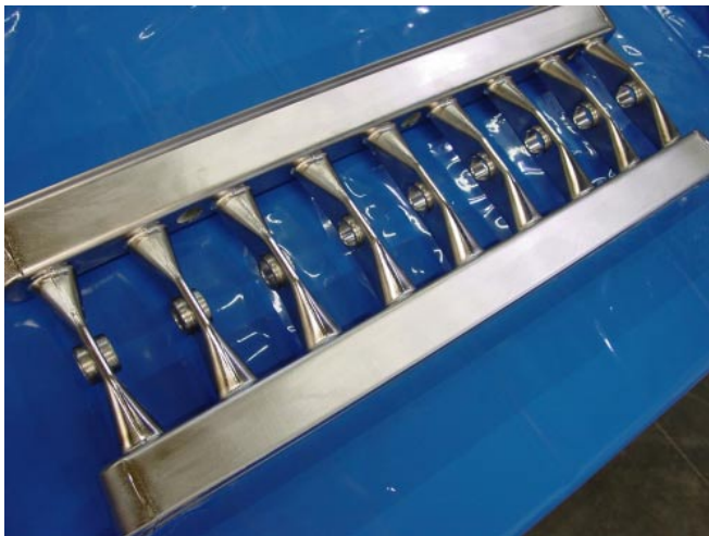
FIG. 18. (Color) Drift-tube structure from bulk niobium welded into one pair of girders during fabrication (courtesy ACCEL).
