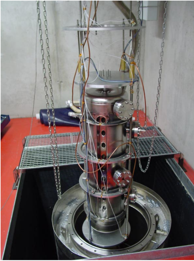
FIG. 27. (Color) Experimental setup for the first cryotest of the CH prototype.
