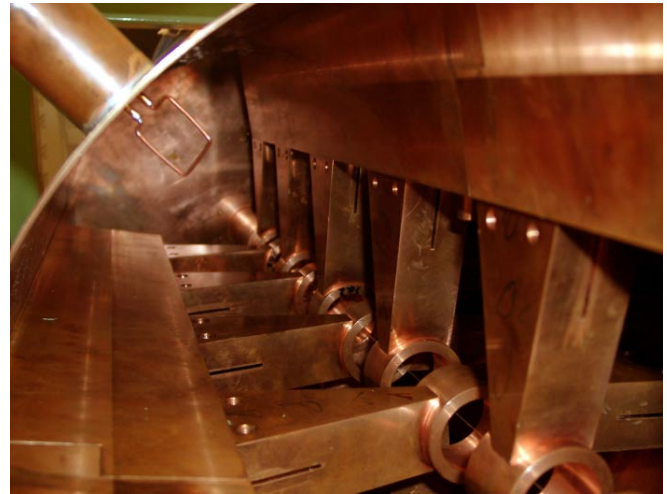
FIG. 16. (Color) The picture shows the location of the inductive coupler in the room temperature copper model. The external Q -value has been varied by changing the loop angle.
