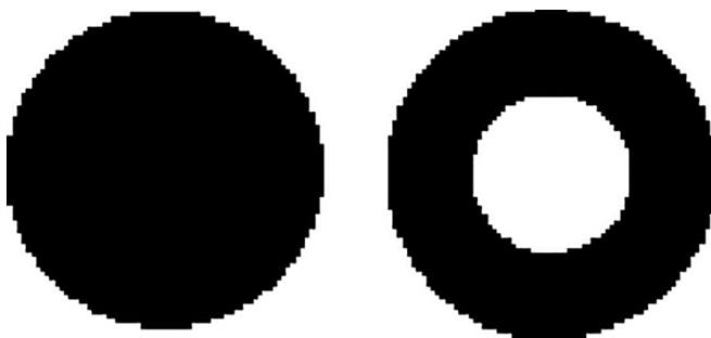
FIG. 8. (Left) Cross section of the optimal configuration for d = 0.64R_{0,3} found numerically for a system with M = 160\,000 spins. The configuration has the shape of a solid 3-ball. This configuration was found to be optimal for all d \leq R_{0,3} . (Right) Cross section of the optimal configuration for d = 1.32R_{0,3} found numerically for a system with M = 160\,000 spins. If the jump length exceeds R_{0,3} the configurations remain isotropic (for d \lesssim 1.4R_{0,3} ) but develop a spherical hole in the center; the radius of the hole grows with increasing d . Note that the outer radius of the configuration is slightly larger than R_{0,3} to ensure that it has unit volume.
