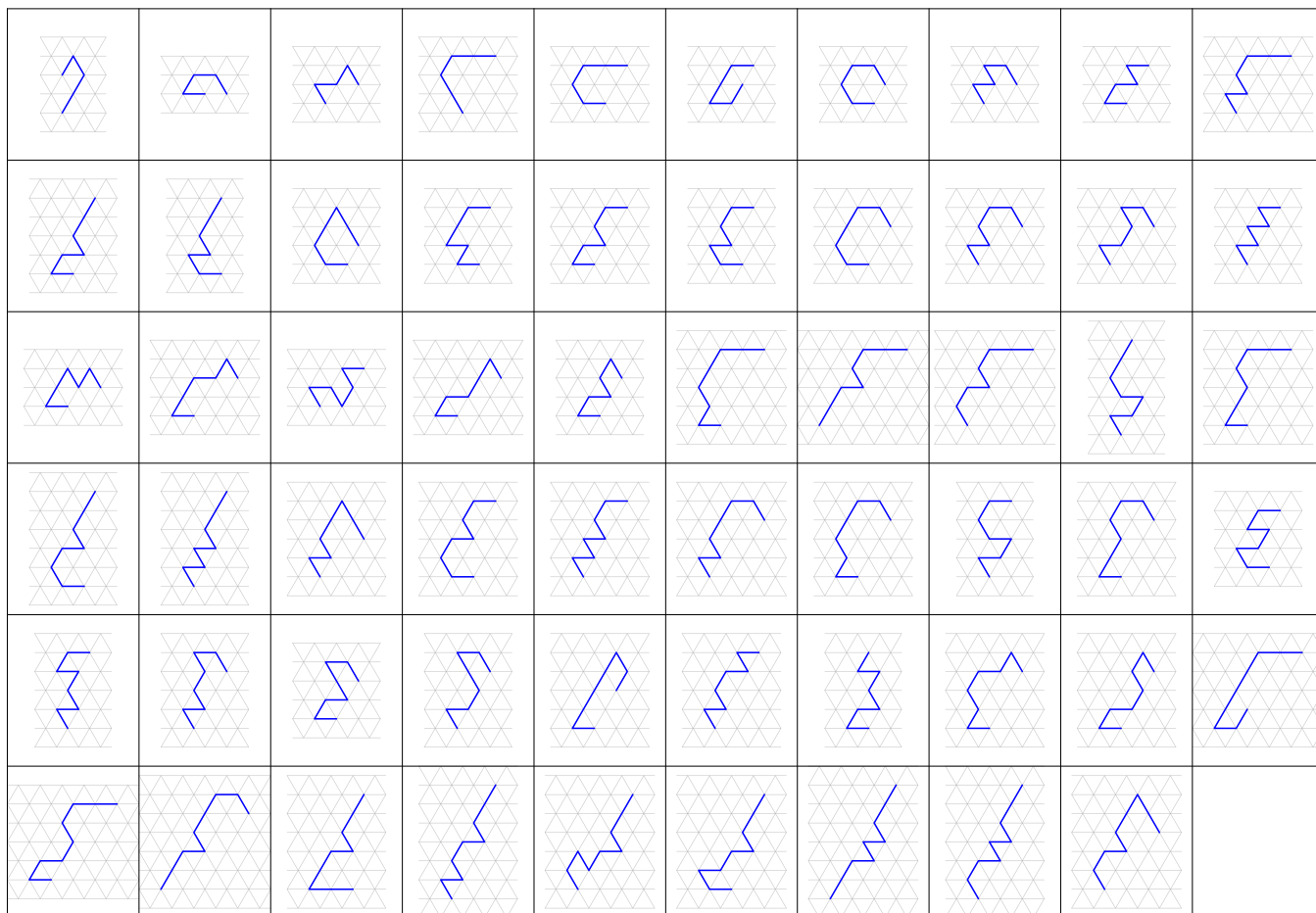
FIG. 36. Self-avoiding partial walks that do not allow a tiling for one or both parts of a seam on an order-6 sphinx frame, and thus can be ruled out immediately.
