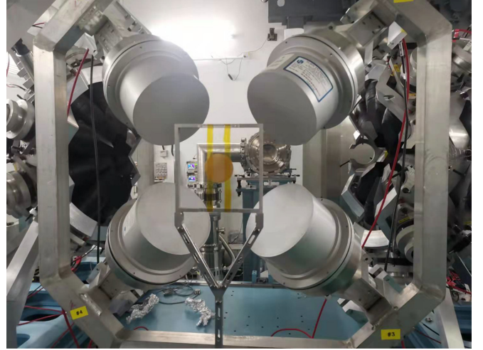
FIG. 3. Photograph of the \text{C}_6\text{D}_6 detector system in the Back-n facility of CSNS; a gold sample is placed in the aluminum sample holder.
