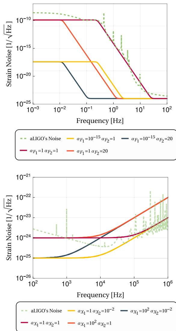
FIG. 4. Force (top row) and sensing noise (bottom row) spectra parametrized by  $\alpha_{F_1}$ ,  $\alpha_{F_2}$ ,  $\alpha_{X_1}$ , and  $\alpha_{X_2}$ . The effect of  $\alpha_{F_1}$  is to rise and lower the nominal noise strength below the cutoff frequency and  $\alpha_{F_2}$  shifts the cutoff frequency. Similarly,  $\alpha_{X_1}$  shifts the cutoff frequency where the sensing noise starts increasing as  $\Omega^2$ , whereas  $\alpha_{X_2}$  shifts the nominal noise level.
