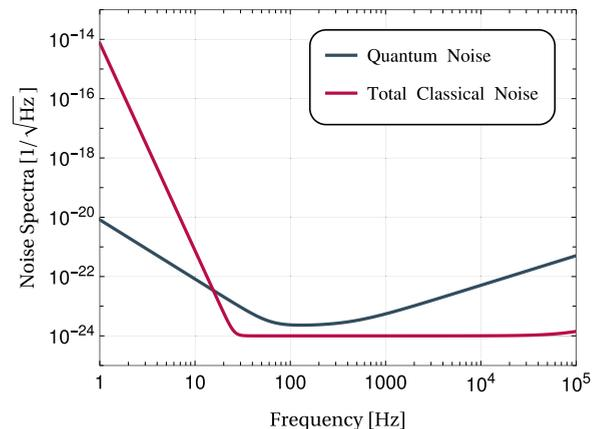
FIG. 7. Modeled noise spectrum for aLIGO.
