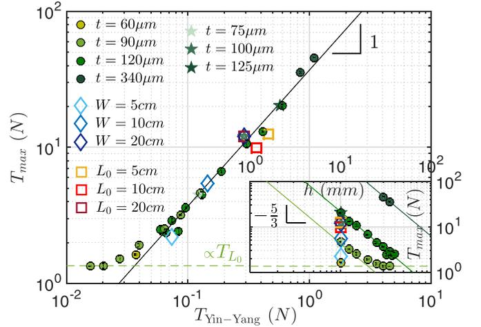
FIG. 8. Experimental measurements of the maximal compressive tangential force  $T_{\max}$  (for different values of  $t$ ,  $W$ ,  $L_0$ , and  $h$  indicated in legends) as a function of the prediction  $T_{\text{Yin-Yang}}$  [Eq. (14)], while the raw data  $T_{\max}(h)$  are plotted in the inset.
