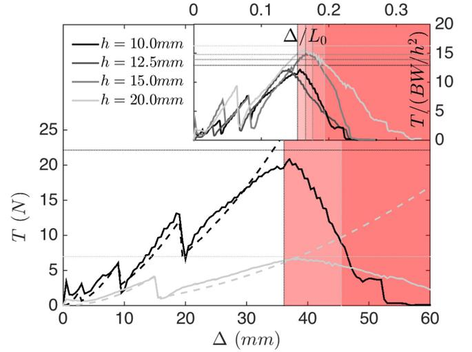
FIG. 5. Tangential force  $T$  as a function of the compression distance  $\Delta$  for a given elastic sheet ( $W = 20$  cm,  $L_0 = 23.5$  cm,  $t = 120$   $\mu\text{m}$ , and  $E = 5$  GPa) at different values of the gap  $h$  in the main panel, while dimensionless data  $T/(BW/h^2)(\Delta/L_0)$  are plotted in the inset. The dashed curves are predictions from Eqs. (6) and (7), while dotted lines are predictions of  $\Delta_{\text{max}}$  and  $T_{\text{max}}$  from Eqs. (13) and (14).
