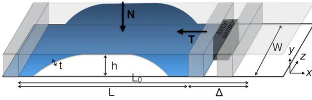
FIG. 1. Scheme of the experiment of compression of a planar sheet under bilateral constraints: the length, width, and thickness of the sheet are  $L_0$ ,  $W$ , and  $t$ ; the confining box is of height  $h$  and length  $L = L_0 - \Delta$ . A force sensor measures the tangential force  $T$ .
