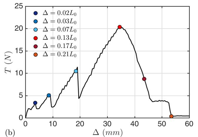
FIG. 2. Tangential force  $T$  as a function of the compression  $\Delta$  for two sets of experimental parameters:  $h = 10$  mm and  $W = 20$  cm; (a)  $L_0 = 10$  cm,  $t = 100$   $\mu\text{m}$ , and  $E = 4$  GPa; (b)  $L_0 = 23.5$  cm,  $t = 120$   $\mu\text{m}$ , and  $E = 5$  GPa. Colored circles in (a) and (b) correspond to pictures in Figs. 3(a) and 3(b), respectively.
