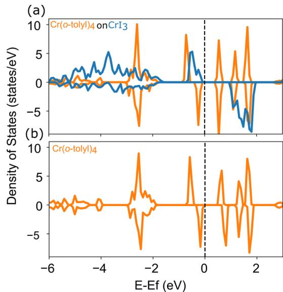
FIG. 6. Density of states for the constrained band calculation of (a)  $\text{Cr}(o\text{-tolyl})_4$  on  $\text{CrI}_3$  and (b) isolated  $\text{Cr}(o\text{-tolyl})_4$ . Both configurations show a doubly occupied  $\text{Cr}(o\text{-tolyl})_4$  orbital near the Fermi level.
