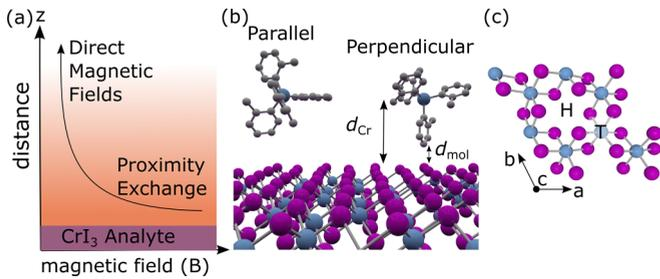
FIG. 1. (a) Sensor-analyte schema to probe magnetic interactions by changing the distance between the MCC sensor and analyte.  $\text{Cr}(o\text{-tolyl})_4$  on  $\text{CrI}_3$  can (b) adopt two configurations with an  $o\text{-tolyl}$  group parallel or perpendicular to the surface at the (c) hollow (H) and top (T) Cr sites on monolayer  $\text{CrI}_3$ .
