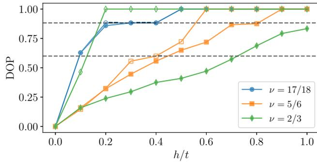
FIG. 3. Degree of polarization (DOP) of an infinite triangular cylinder of  $L_y = 6$  as a function of the external magnetic-field  $h$  at different filling factors  $\nu$  at  $J/t = 0$  and at zero temperature. Filled (empty) symbols correspond to the case  $V/t = 0$  ( $V/t = 6$ ). The dashed line indicates the polarization plateau expected for the magnetic polaron gas at  $\nu = 17/18, 5/6$ .
