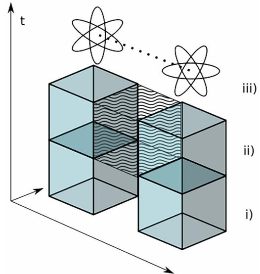
FIG. 4. Simplified space-time diagram for generating a logical Bell state between two surface codes. Each solid cube represents  $D$  cycles of syndrome extraction where  $D$  is the code distance. (i) Initialization of surface code qubits in the  $|00\rangle_L$  state. (ii) Lattice merging with shared entanglement represented by the wavy cube connecting the two code patches. (iii) Lattice splitting, which requires a single round of syndrome extraction.
