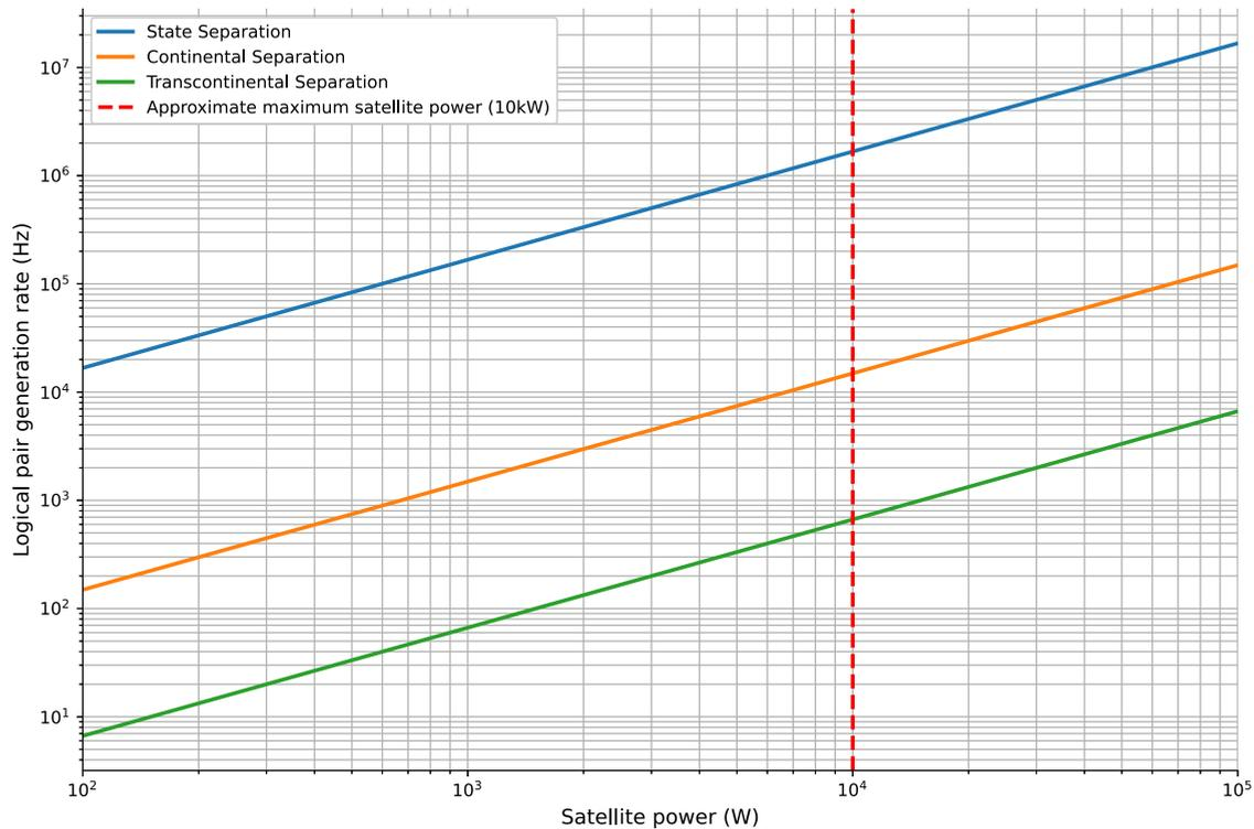
FIG. 5. Rate at which logical surface code Bell pairs can be generated versus the available satellite power [Eq. (26)] for three different distance ratings (Table I). The vertical dashed line indicates the approximate maximum power of a commercial satellite [29].
