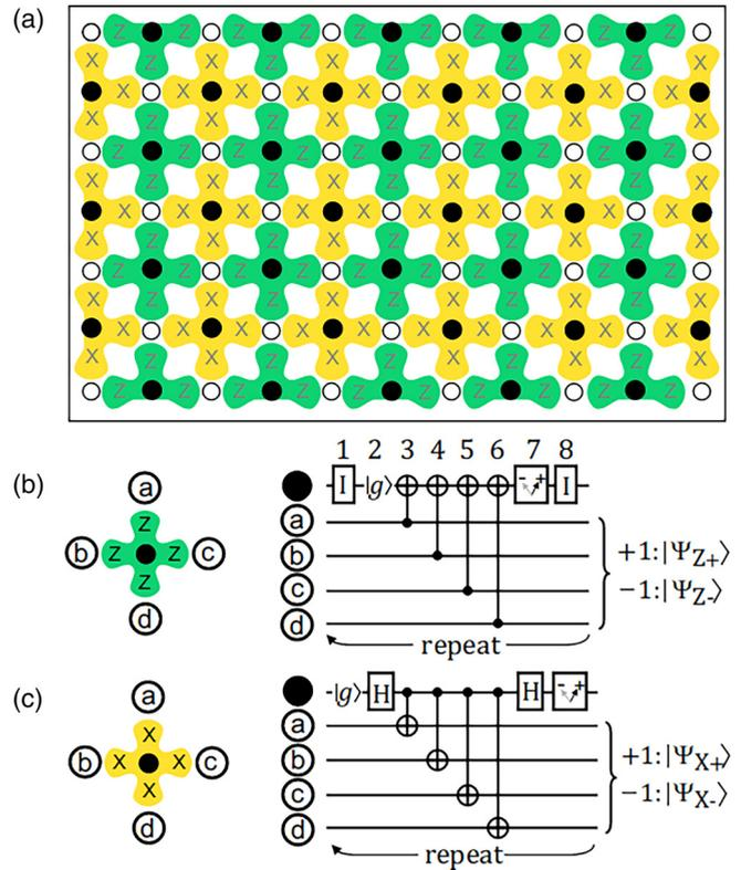
FIG. 2. (a) Top-down schematic of the surface code. The white (black) circles are the data (syndrome) qubits and the green (yellow) clover structures are the vertex (face) plaquettes. (b), (c) Syndrome extraction circuits for the two types of stabilizer generators for the surface code, respectively. Figure reproduced from Horsman *et al.* [15].
