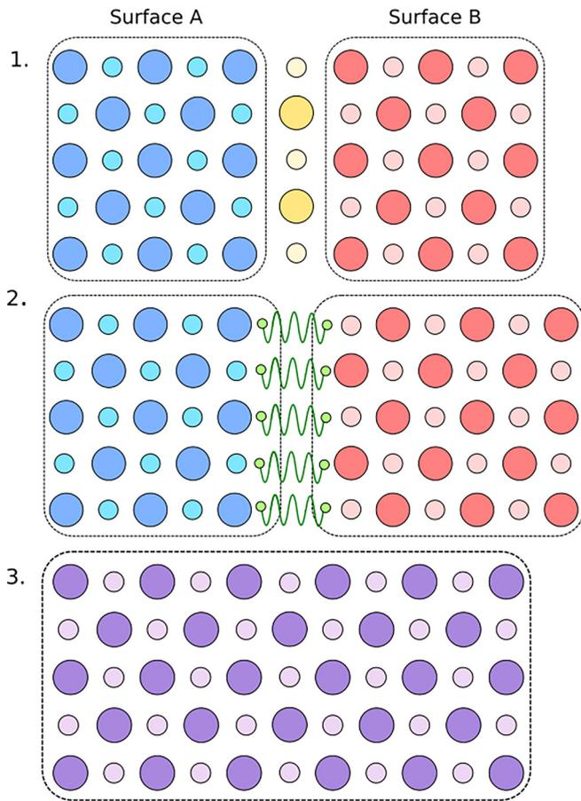
FIG. 3. Illustration of lattice surgery between two spatially separated surface codes  $A$  and  $B$ . (1) A buffer of syndrome and data qubits is initialized between the two surfaces for continuity of the qubit pattern. (2) The buffer qubits are merged into surface  $B$  and Bell pairs are delivered for each qubit pair on the boundary. (3) The syndrome extraction cycle of the code proceeds as normal. This joins the two patches into a single code.
