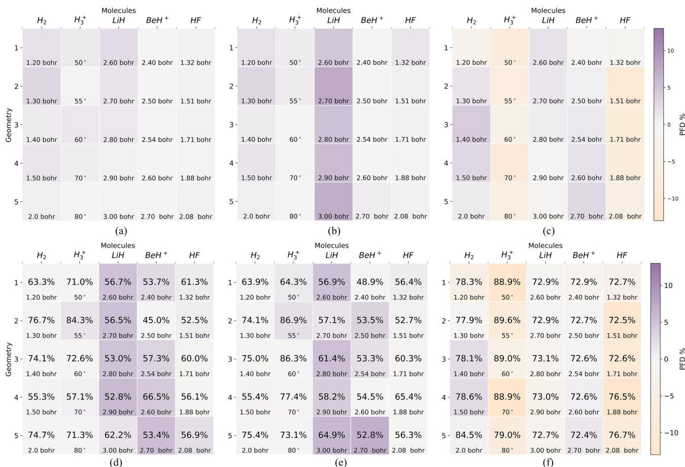
FIG. 5. Heat map plot showing the circuit depth compression observed in the corresponding HHL variant with respect to quantum circuit depth of the HHL algorithm, as well as the PFD of correlation energies obtained from (a) HHL, (b) PerturbedHHL, (c) AdaptHHL, (d) HHLite, (e) PerturbedHHLite, and (f) AdaptHHLite schemes for the set of molecules considered. The text inside the grid shows the circuit depth compression in percentage along with the geometry of the molecule. The color gradient represents the PFD with respect to LCC calculation on a traditional computer. We note that for all of our numerical results for AdaptHHL and AdaptHHLite, we set \tilde{d}_{\min} to d_{\min} , as mentioned in Sec. II B 2 a.
