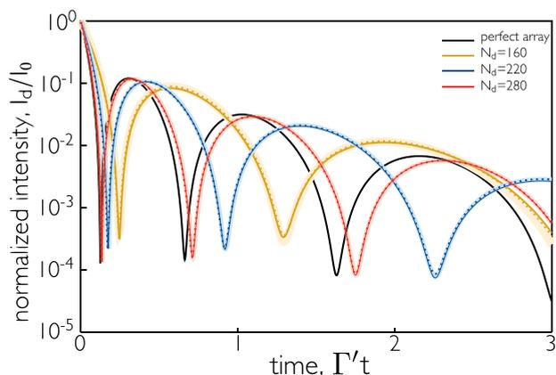
FIG. 3. Light intensity after switching off a square pulse propagating through an imperfectly filled array with 300 sites,  $\Gamma_{1D}/\Gamma' = 0.08$  and  $\Delta = 0.3\Gamma'$ . In each run, there are  $N_d$  qubits, with  $N_d \leq N$ . The results of the imperfectly filled arrays (solid lines), the perfect arrays of  $N_d$  qubits (thick light lines), and the Bessel expansion of Eq. (5) with  $b = N_d\Gamma_{1D}/2$  (dotted lines) are in agreement.
