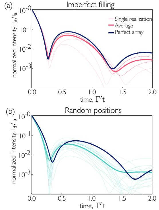
FIG. 5. Impact of position disorder on transients for a low qubit number. (a) Transients produced by five atoms positioned at random in an array of ten sites with lattice constant  $k_{1D}d = \pi/2$ . (b) Transients produced by five atoms with random positions.  $\Gamma_{1D}/\Gamma' = 2.5$  and  $\Delta/\Gamma' = 0.5$  for both plots. To get the average curves, 100 realizations were used.
