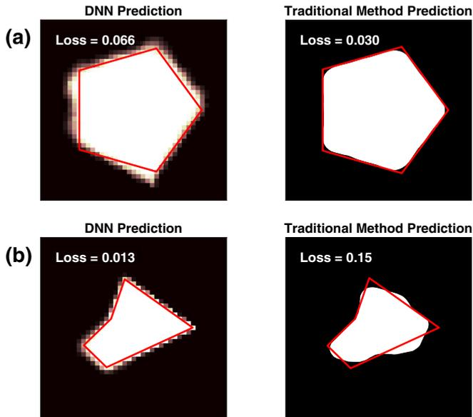
FIG. 9. Reconstructions from the DNN and the traditional method [15] for (a) a regular pentagon and (b) a concave pentagon.
