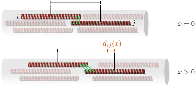
FIG. 4. Deformation of cross links connecting two microtubules  $i$  and  $j$ . The rate of deformation depends on the distance between the two microtubules, whose respective centers of mass undergo affine displacement.
