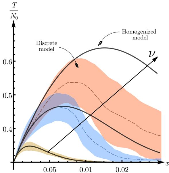
FIG. 3. Comparison of our homogenized model with the discrete finite-element model of [32]. Tension-strain curves  $T/N_0$  vs  $x$ , for  $\nu = 0.01, 0.04, 0.07$ , and  $0.1$ . Solid lines correspond to the homogenized model. Colored streaks show the mean and standard deviation for 14 simulations of the discrete model for each value of  $\nu$ .
