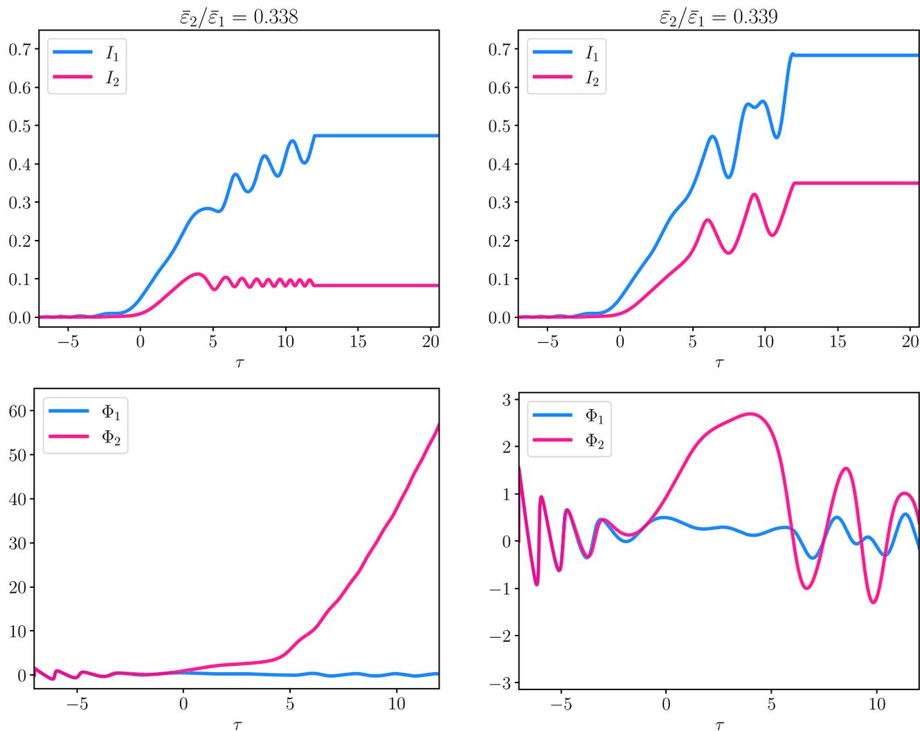
FIG. 9. The effective actions  $I_1, I_2$  (top subplots) and the phase mismatches  $\Phi_1, \Phi_2$  (bottom subplots) vs slow time  $\tau = \sqrt{\alpha_1}t$  obtained by solving the weakly nonlinear reduced dynamical equations (38)–(41). The parameters used in the simulations are the same as in Figs. 1(a), 2, and 3 except for parameter  $\bar{\epsilon}_2$ , which is equal to  $\bar{\epsilon}_2 = 0.338\bar{\epsilon}_1$  (left side) and  $\bar{\epsilon}_2 = 0.339\bar{\epsilon}_1$  (right side).
