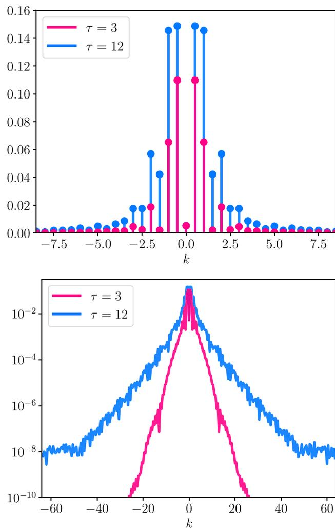
FIG. 5. The spectrum of the harmonics of the ion fluid velocity  $u(x, \tau)$  in  $k$  space obtained by solving the fully nonlinear equations (1)–(3) at  $\tau = 3$  (pink line) and  $\tau = 12$  (blue line) in linear (top subplot) and logarithmic (bottom subplot) scales. The parameters used in the simulations are the same as in Figs. 1(a), 2, 3, and 4.
