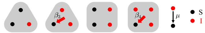
FIG. 1. Schematic representation of simplicial susceptible-infected-susceptible ( s -SIS) model. Black dots represent susceptible nodes, red dots represent infected nodes, and the grey area represents hyperedges. The contagion along a hyperedge occurs if and only if exactly one node is susceptible and all the other nodes are infected. If the condition is met, the susceptible node is turned to the infected state with rate \beta_d , where d is the size of the hyperedge. If the hyperedge is immunized, the contagion through the hyperedge does not occur. Additionally, the recovery process S \rightarrow I is defined identically to the traditional susceptible-infected-susceptible (SIS) model.
