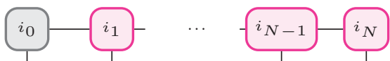
FIG. 6. Diagrammatic representation of a right-canonical MPS, where the OC is situated at the left of the system (black) and the rest of the bins are right normalized (magenta).
