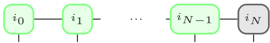
FIG. 5. Diagrammatic representation of a left-canonical MPS, where the OC is situated at the right of the system (black) and the rest of the bins are left normalized (green).
