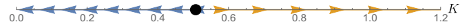
FIG. 2. The RG flow of the 2d Ising model without a magnetic field h = 0 , when the square interactions K'_3 are negligible (13). The fixed point K_c = J/T_c = 0.507 is depicted and is unstable.
