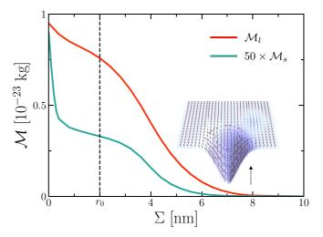
FIG. 3. Curvature-induced mass  $\mathcal{M}$  as a function of the collective coordinate  $\Sigma$  in physical units.  $\Sigma$  represents the distance between the center of the defect and the center of the skyrmion.  $\mathcal{M}_l$  ( $\mathcal{M}_s$ ) denotes the mass for the large (small) radius skyrmion, and the vertical dashed line indicates the defect width  $r_0$ .
