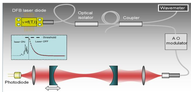
FIG. 3. Scheme of the CRD spectrometer. The different components include a distributed feedback diode laser (DFB), an optical isolator, a fiber coupler, an acousto-optic (AO) modulator and a photodiode. The inset shows the time dependence of the light intensity measured by the photodiode: after a build-up period, the light intensity reaches a threshold value which triggers the switch off of the AO modulator. The ring down time is then measured from the exponential decay of the light intensity.
