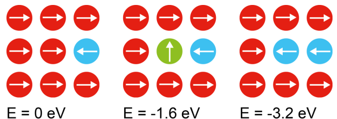
FIG. 8. The demagnetization energy is reduced by 1.6 and 3.2 eV upon rotation of the center disk by 90^\circ and 180^\circ , respectively.
