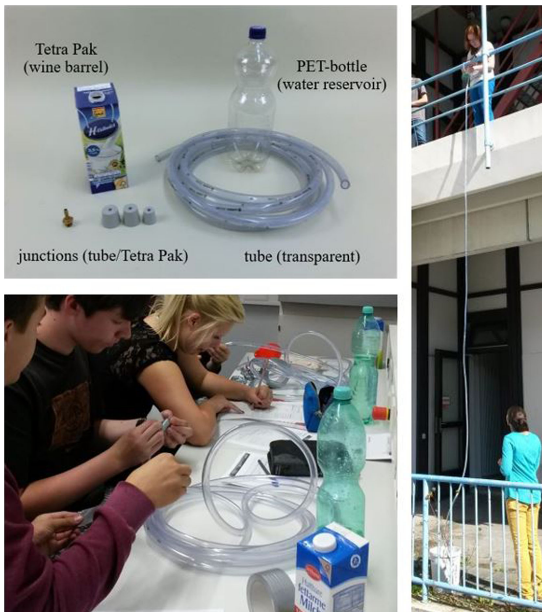
FIG. 4. Hands-on experiment on the bursting of a wine barrel according to Blaise Pascal [122]. Because of the necessary height difference (several meters), part of the activity was carried out outside the building.
