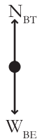
FIG. 17. Free body diagram for the bowling ball in the bowling ball free body diagram question.
