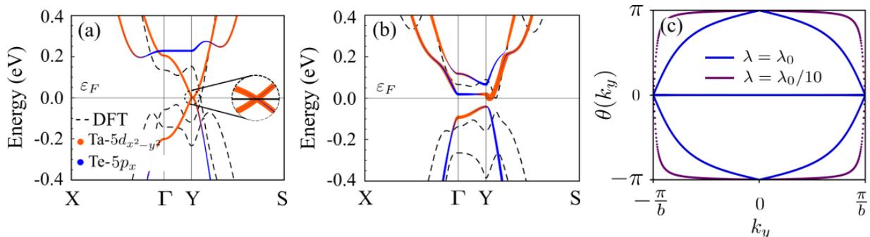
FIG. 3. TB model for monolayer TaRhTe<sub>4</sub>. Band structures obtained from the four-orbital TB model for (a) without and (b) with SOC along with the orbital contributions. The DFT bands are shown with black dashed lines for comparison. (c) Wilson loop spectra for the TB model (blue curve), and for the model where the SOC terms are scaled down to 10% of the real values (purple color).
