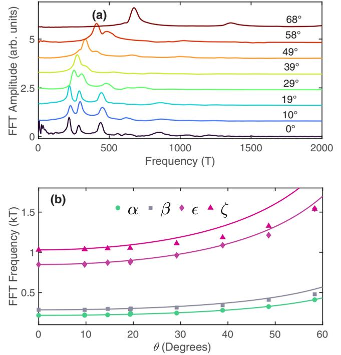
FIG. 3. (a) Angular dependence of the Fourier transform amplitude (offset for clarity) vs frequency of the background subtracted torque signal vs  $1/H$  for the  $\text{CsTi}_3\text{Bi}_5$  torque measurement. (b)  $1/\cos(\theta)$  fitting for the angular dependence of the Fourier transform frequency in the for the observed fundamental frequency peaks.
