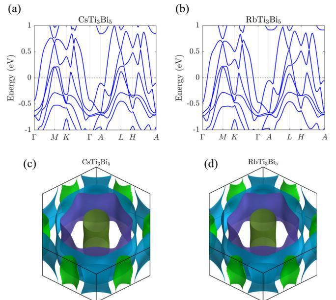
FIG. 7. (a) and (b) are the band structures of  $\text{CsTi}_3\text{Bi}_5$  and  $\text{RbTi}_3\text{Bi}_5$ , respectively, with spin-orbital coupling. (c) and (d) are the respective Fermi surfaces. Both the band structure and Fermi surface of  $\text{RbTi}_3\text{Bi}_5$  are very similar to those of  $\text{CsTi}_3\text{Bi}_5$ . Notice that only the green Fermi surfaces around the  $M-L$  lines are hole pockets while others are electron pockets.
