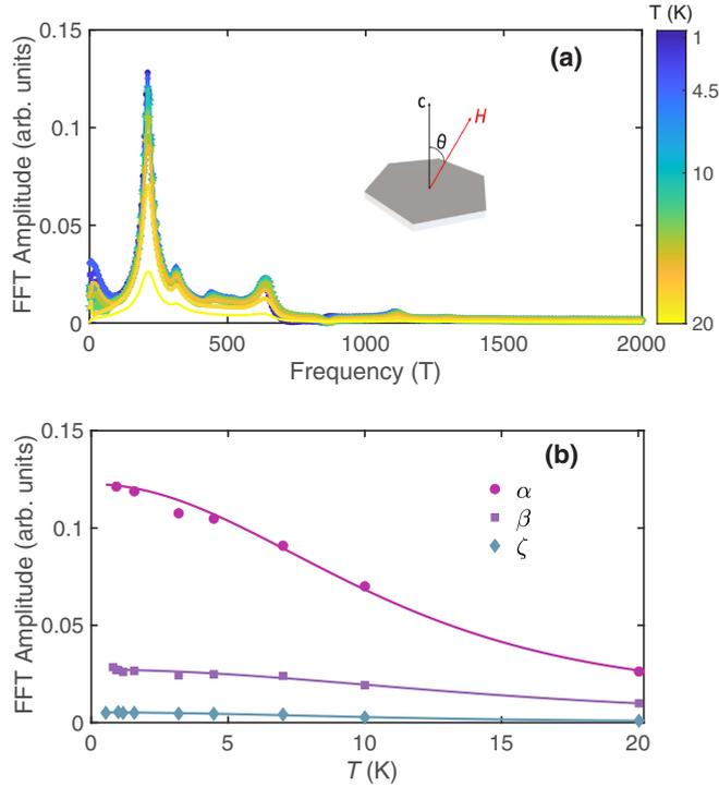
FIG. 4. (a) Temperature dependence of the Fourier transform amplitude vs frequency, at  $\theta = 40$  degrees, of the background subtracted torque signal vs  $1/H$  for  $\text{RbTi}_3\text{Bi}_5$ . The inset shows how we measure the angle relative to the  $ab$  plane. (b) Lifshitz-Kosevich fitting for the temperature dependence of the Fourier transform amplitudes for the observed fundamental frequency peaks in  $\text{RbTi}_3\text{Bi}_5$ .
