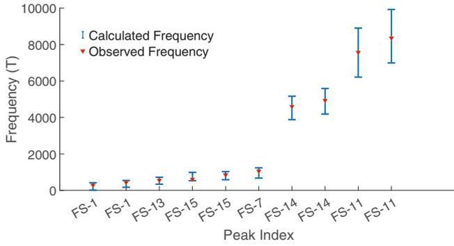
FIG. 8. Calculated and observed Fourier transform peak frequencies for  $\text{CsTi}_3\text{Bi}_5$  are shown with the Fourier peak index from the DFT calculations on the  $x$  axis. The frequency dispersion per peak was calculated by tuning the Fermi level from  $-100$  meV to  $100$  meV, with the error bars being the  $\pm 100$  meV values of the Fermi level.
