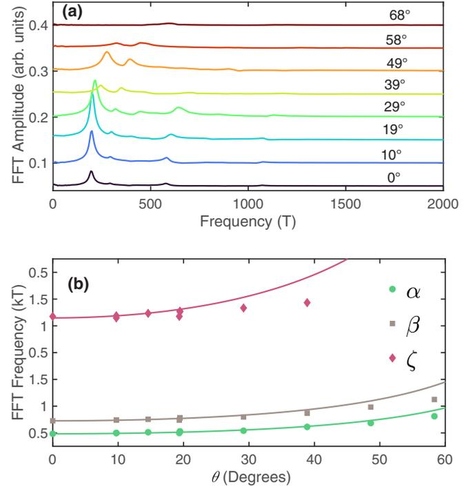
FIG. 5. (a) Angular dependence of the Fourier transform amplitude (offset for clarity) vs frequency of the background subtracted torque signal vs  $1/H$  for  $\text{RbTi}_3\text{Bi}_5$ . (b)  $1/\cos(\theta)$  fitting for the angular dependence of the Fourier transform frequency for the observed fundamental frequency peaks in  $\text{RbTi}_3\text{Bi}_5$ .
