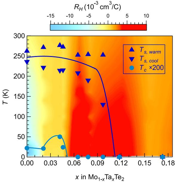
FIG. 5. Temperature-doping phase diagram of  $\text{Mo}_{1-x}\text{Ta}_x\text{Te}_2$ . The upward (downward) blue triangles represent  $T_s$  defined from the temperature-dependent resistivity data measured during warm-up (cool-down). The solid cyan circles represent  $T_c$ . The solid curves are guides for the eyes. The color contour denotes the temperature dependence of Hall coefficient  $R_H$  at different doping levels.
