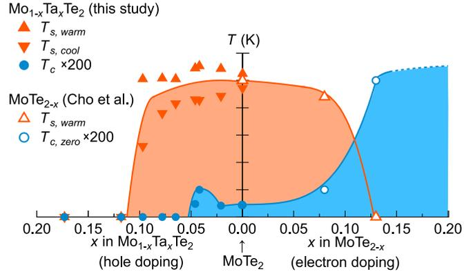
FIG. 6. Temperature-doping phase diagram of hole-doped and electron-doped  $\text{MoTe}_2$ . The hole-doping data (solid symbols) are our findings of  $\text{Mo}_{1-x}\text{Ta}_x\text{Te}_2$ , as shown in Fig. 5, while the electron-doping data (open symbols) are adapted from the findings of Te-deficient  $\text{MoTe}_{2-x}$  from Cho *et al.* [27].
