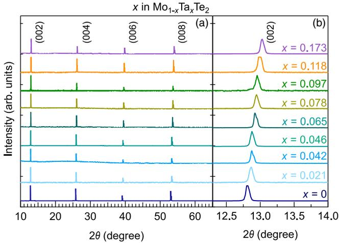
FIG. 1. (a) x-Ray diffraction (XRD) spectra of single crystals of  $\text{Mo}_{1-x}\text{Ta}_x\text{Te}_2$ . The peaks of  $(00L)$  are indexed in the figure. (b) Enlarged XRD spectra near the peak of  $(002)$ . The  $(002)$  peak shifts progressively toward a higher diffraction angle  $2\theta$  when  $x$  increases.
