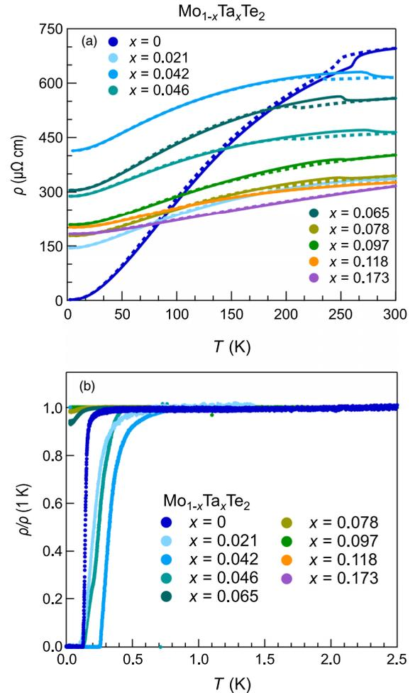
FIG. 2. (a) Temperature dependence of resistivity  $\rho(T)$  of  $\text{Mo}_{1-x}\text{Ta}_x\text{Te}_2$  at zero magnetic fields. The warm-up (cool-down) data are plotted as solid (dashed) curves. (b) Low-temperature  $\rho(T)$  normalized to the value of  $\rho(1\text{ K})$ , displaying the superconducting transitions.
