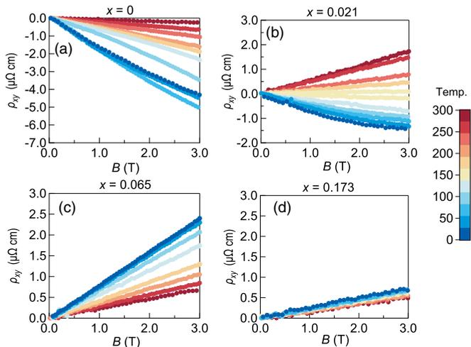
FIG. 3. Magnetic field dependence of Hall resistivity  $\rho_{xy}(B)$  of  $\text{Mo}_{1-x}\text{Ta}_x\text{Te}_2$  with (a)  $x = 0$ , (b)  $x = 0.021$ , (c)  $x = 0.065$ , and (d)  $x = 0.173$  collected during warm-up. The color scale at the right indicates the measured temperature.
