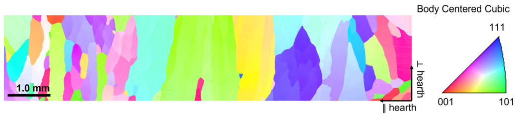
FIG. 6. Electron backscatter diffraction (EBSD) orientation maps of as-cast Fe-Ga with 65-ppm Ce. The top of the image corresponds to the top of the sample, while the bottom is the surface nearest the hearth of the arc melter. Large grains are visible across the vertical extent of the sample, indicating significant effects of cooling direction.
