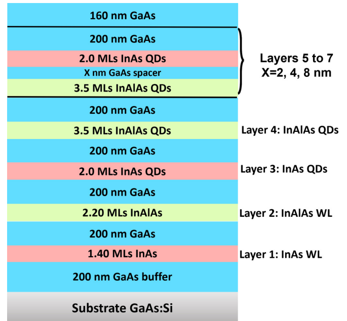
FIG. 1. Schematic structure of the sample grown by molecular beam epitaxy for the X-STM experiments.
