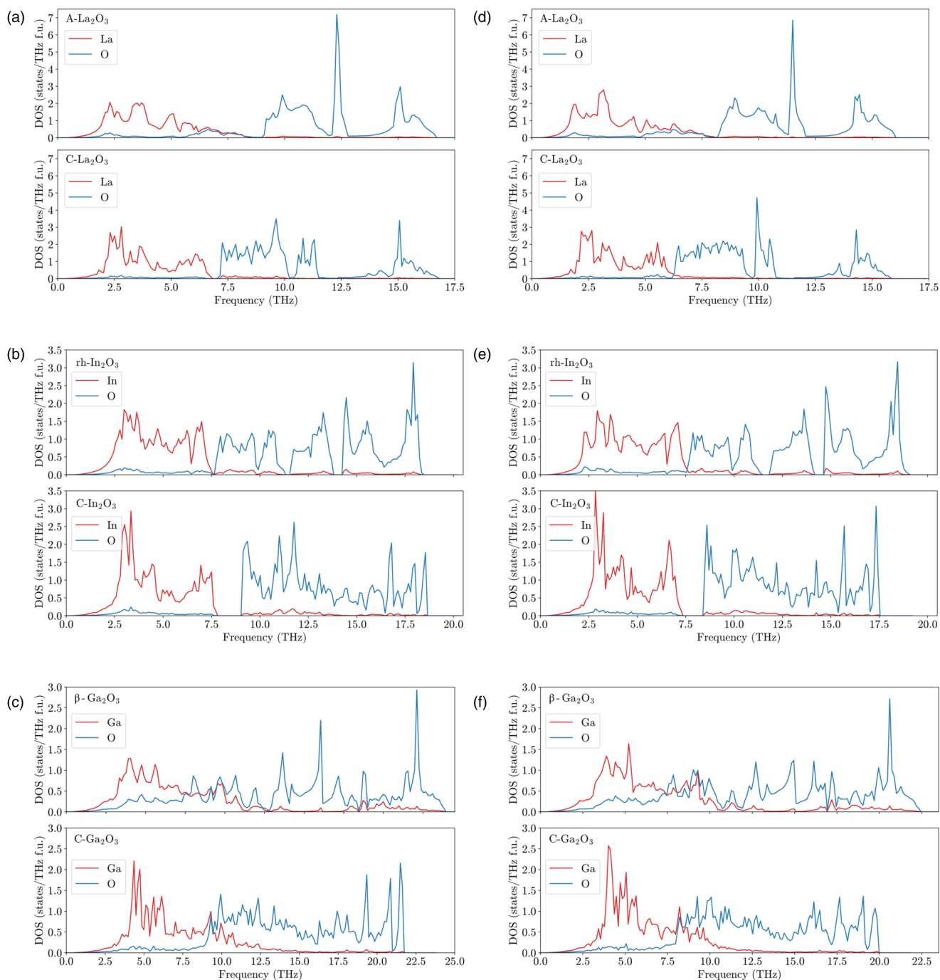
FIG. 4. Phonon density of states for ground state and metastable structures of (a) \text{La}_2\text{O}_3 , (b) \text{In}_2\text{O}_3 , and (c) \text{Ga}_2\text{O}_3 calculated using LDA, and bixbyite (d) \text{La}_2\text{O}_3 , (e) \text{In}_2\text{O}_3 , and (f) \text{Ga}_2\text{O}_3 calculated using GGA PBE.
