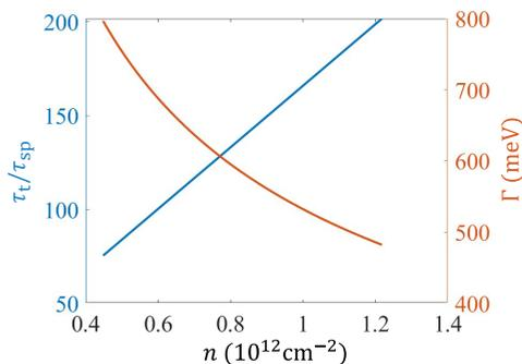
FIG. 29. Plot of calculated ratio of the transport time  $\tau_t$  to the single-particle relaxation time  $\tau_{\text{sp}}$  and the single particle level broadening  $\Gamma$  as a function of density for the InSb sample from the Bakkers group in Eindhoven. Here we consider only 3D background impurities distributed in the 2D InSb quantum well with the width  $a = 80$  nm.
