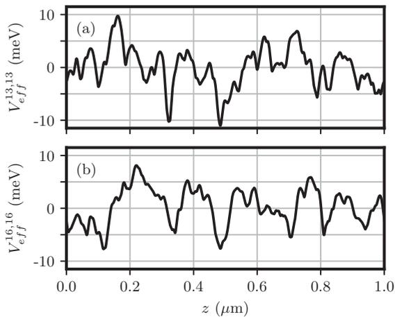
FIG. 23. Effective disorder potential  $V_{\text{dis}}(z) = V_{\text{eff}}^{\alpha,\alpha}(z)$  for a system with the bottom of the  $\alpha$  subband tuned near the Fermi level, where (a)  $\alpha = 13$ , which corresponds to a back gate voltage  $V_{\text{BG}} = -2.78$  V, and (b)  $\alpha = 16$ , which corresponds to  $V_{\text{BG}} = -1.90$  V. The side gates are at zero voltage,  $V_L = V_R = 0$ .
