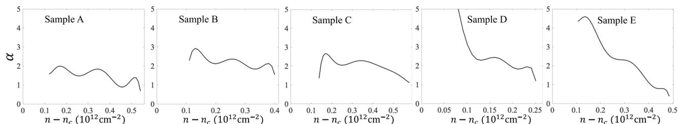
FIG. 27. Numerically extracted exponent obtained through  $\alpha = \frac{d \ln \mu}{d \ln n}$  from the InAs transport data from the Copenhagen group of Krogstrup.
