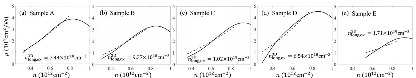
FIG. 10. Same as Fig. 6, but considering only remote impurities distributed three dimensionally (i.e., 3D long-range impurities) in the dielectric layer of thickness  $a_{\text{oxide}} = 8$  nm located 10 nm away from the interface of the quantum well.
