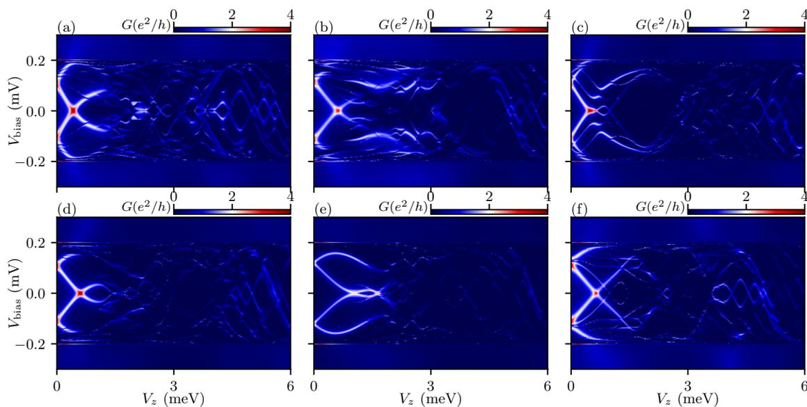
FIG. 16. Conductance as a function of the applied Zeeman field and bias voltage in the presence of six different disorder realizations with  $\sigma_\mu = 3$  meV. Only these six disorder configurations (out of 120) support a low-field ZBCP (at either the left or the right end of the system). The chemical potential is  $\mu = 3$  meV, while the other parameters are the same as in Fig. 15.
