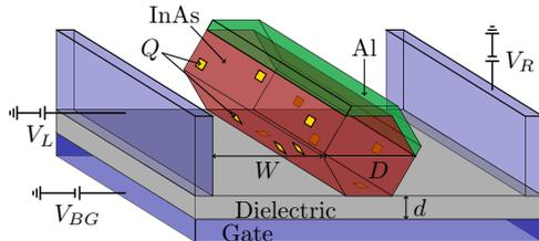
FIG. 21. Schematic representation of a hybrid device consisting of a semiconductor (InAs) nanowire (red) of diameter  $D$  proximity coupled to a thin superconductor (Al) layer (green). Metallic gates (blue) control the electrostatic environment. Charge impurities (yellow squares), each carrying charge  $Q$ , are randomly placed on the facets of the nanowire that are not covered by Al and produce a nonuniform potential along the length of the device.
