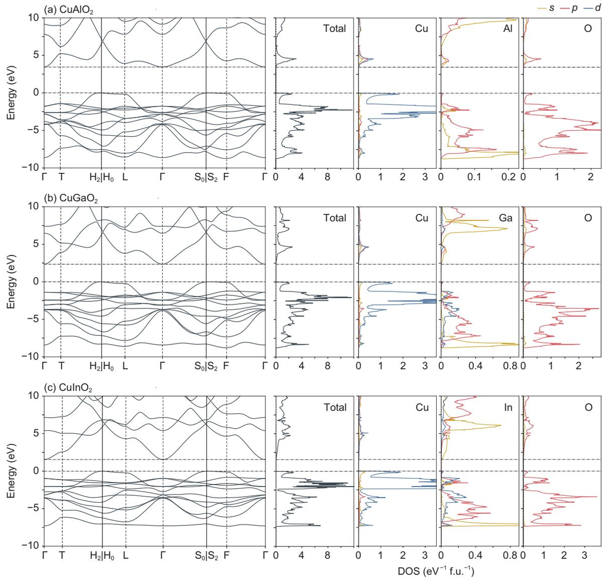
FIG. 2. Band structures, total DOSs, and the DOSs projected on each of the atomic site and orbital for (a)  $\text{CuAlO}_2$ , (b)  $\text{CuGaO}_2$ , and (c)  $\text{CuInO}_2$ . The band paths are determined using the seekpath code [52]. The VBMs are set to zero energies, which are indicated by the horizontal dashed lines as well as the CBMs.
