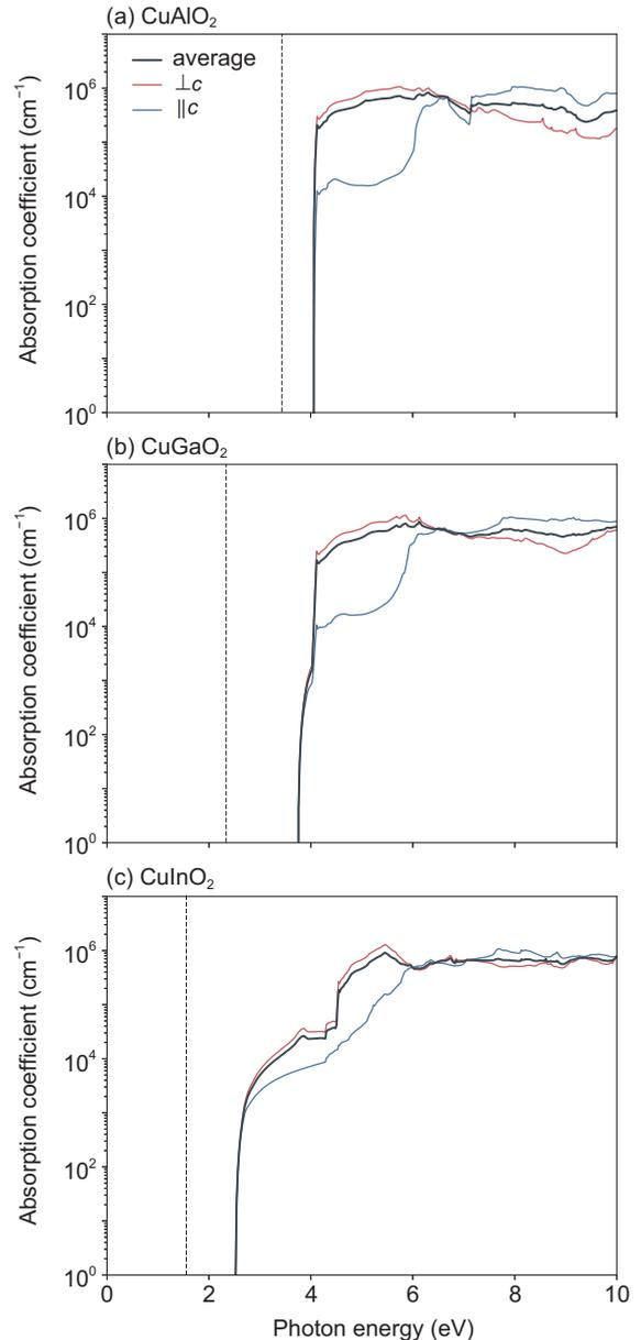
FIG. 3. Absorption spectra for (a)  $\text{CuAlO}_2$ , (b)  $\text{CuGaO}_2$ , and (c)  $\text{CuInO}_2$ . The black, red, and blue curves represent the spherically average and the components for the polarization perpendicular and parallel to the  $c$  axis, respectively. The dashed line indicates the minimum (indirect) band gaps.
