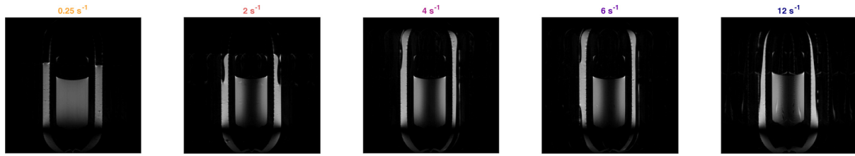
FIG. 11. MRI images of the rheo-NMR cell with 2.5 mm gap after shearing for 10 min at various rates. (Sequence RARE 256 \times 256 , FOV = 5 cm \times 5 cm, RARE factor = 32, TE = 72 ms, TR = 1.5 s, NA = 1, measuring time = 24 s).
