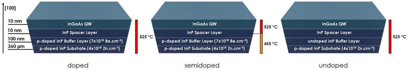
FIG. 1. Layer structure of the  $\text{In}_{0.53}\text{Ga}_{0.47}\text{As}$  quantum wells grown on InP (001) by molecular beam epitaxy. The doping of the InP buffer layer and the occurrence of an interruption step during the growth of the heterostructure to change the sample temperature allows growth of quantum wells with different hole doping levels. Depending on the degree of Be diffusion during the growth, the samples are labeled *doped*, *semidoped*, and *undoped*.
