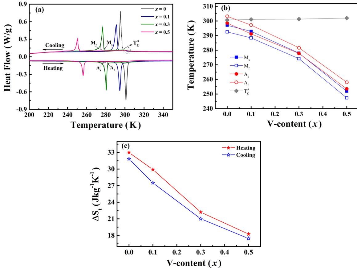
FIG. 1. (a) DSC curves during heating and cooling for  $\text{Ni}_{51-x}\text{Mn}_{33.4}\text{In}_{15.6}\text{V}_x$ . (b) Characteristic temperatures and (c) total entropy change during the structural transition extracted from the DSC curves as a function of the V content.
