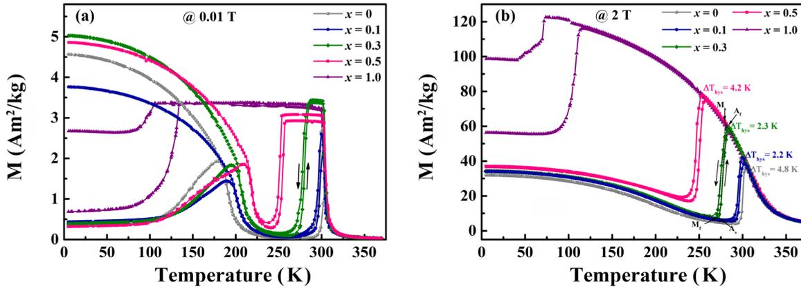
FIG. 3. ZFC and FC  $M$ - $T$  curves for an applied field of (a) 0.01 T and (b) 2 T of  $\text{Ni}_{51-x}\text{Mn}_{33.4}\text{In}_{15.6}\text{V}_x$  alloys. The characteristic temperatures- $M_s$ ,  $M_f$ ,  $A_s$ , and  $A_f$  are indicated and  $\Delta T_{\text{hys}}$  are listed.
