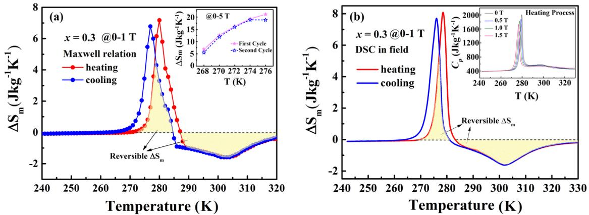
FIG. 5. Magnetic entropy change ( $\Delta S_m$ ) as a function of temperature for the heating and cooling processes determined by (a) the Maxwell relation and (b) the specific heat in field (shown in the inset) for sample with  $x = 0.3$ . The yellow area represents the reversible part of the entropy change. The inset of Fig. 3(a) shows  $\Delta S_m$  under two magnetic cycles with a field change of 0–5 T.
