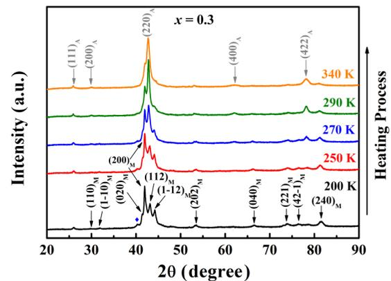
FIG. 8. Temperature dependence of the XRD patterns for the sample with  $x = 0.3$  for increasing the temperatures. The crystal indices of austenite and martensite are indicated. The minor peak (blue diamond) corresponds to the satellite reflections generated by a structural modulation.
