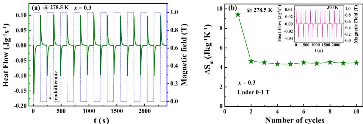
FIG. 6. (a) Calorimetric curves (solid line) obtained under isothermal conditions with a cyclic application/removal of the magnetic field (blue dash line) at 278.5 K. (b)  $\Delta S_m$  in 10 field cycles of 0–1 T. The inset is the calorimetric curves under cyclic fields at 300 K.
