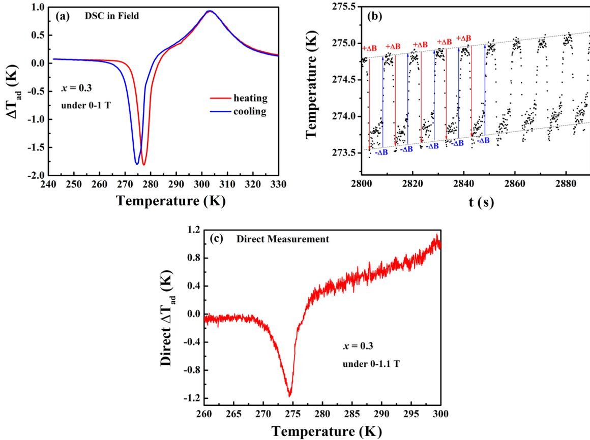
FIG. 7. (a) Temperature dependence of  $\Delta T_{ad}$  from DSC measurements for  $\Delta B = 1$  T. (b) Temperature versus time during direct  $\Delta T_{ad}$  measurements in sweep mode for  $\Delta B = 1.1$  T. (c)  $\Delta T_{ad}$  versus temperature evolution during the temperature sweep.
