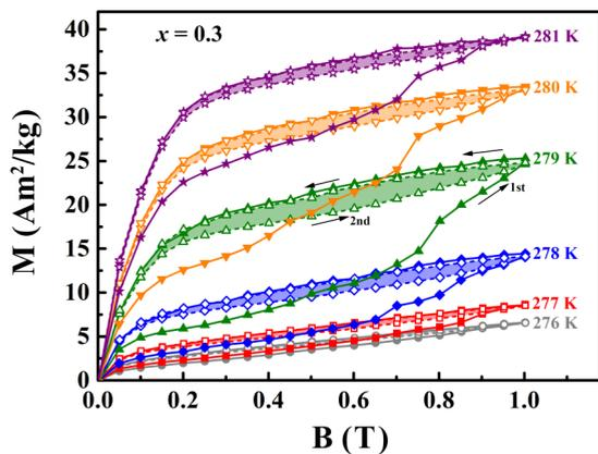
FIG. 4. Isothermal magnetization curves as a function of the applied magnetic field around  $T_i$  in the field range of 0–1 T under two magnetic cycles for the sample with  $x = 0.3$ . The measurements are performed in the heating process.
