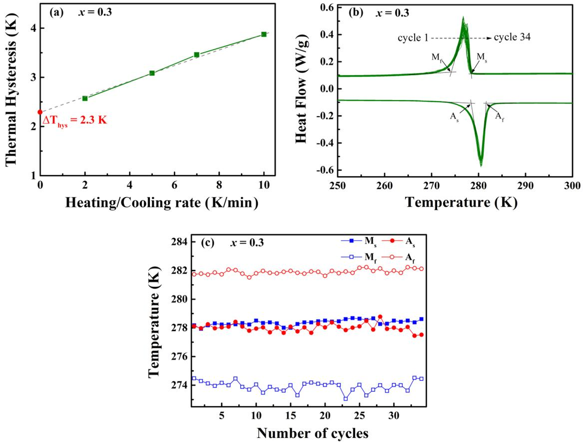
FIG. 2. (a) Thermal hysteresis obtained from DSC curves for  $\text{Ni}_{51-x}\text{Mn}_{33.4}\text{In}_{15.6}\text{V}_x$  measured at different sweep rates. (b) DSC curves and (c) characteristic transformation temperatures under 34 thermal cycles for sample with  $x = 0.3$ .
