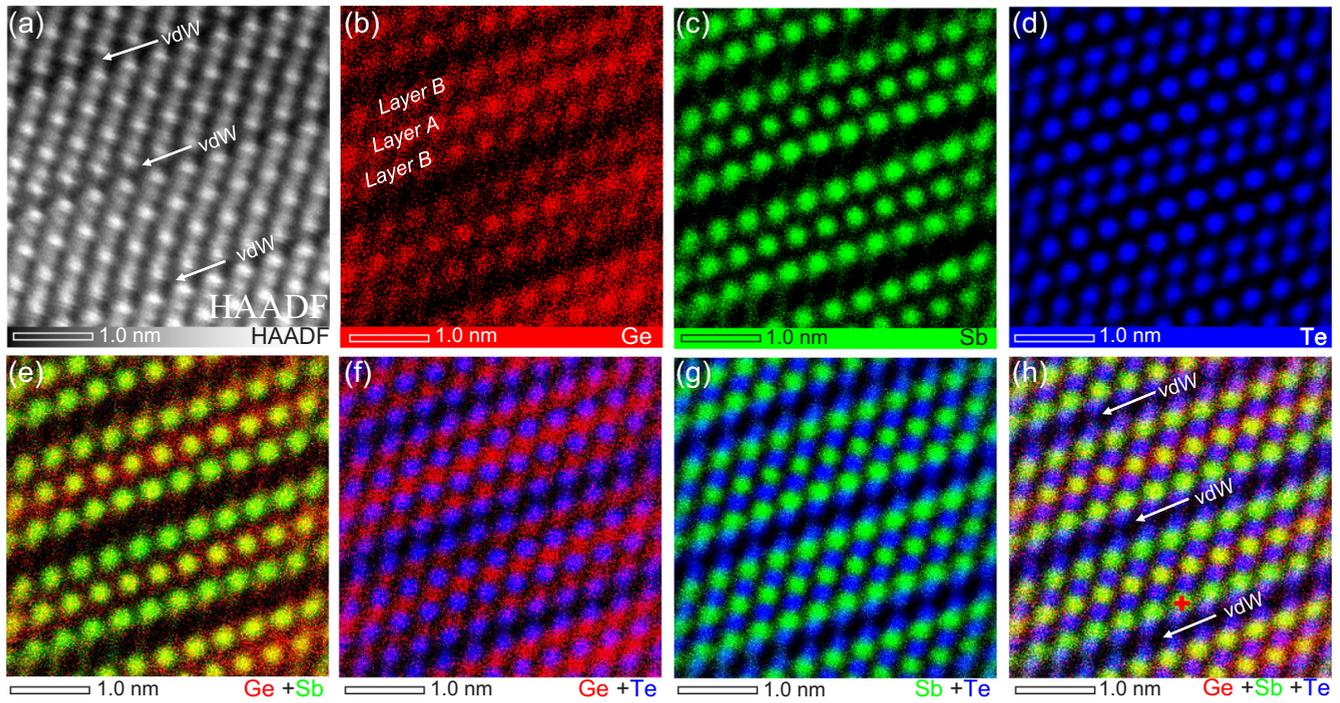
FIG. 1. Structural and chemical identifications in a  $\text{Ge}_1\text{Sb}_2\text{Te}_4$  crystallite with HEX phase, projected along the  $[11-20]$  direction. (a) HAADF-STEM image of the transition region. The arrows mark the vdW gap between two blocks. (b)–(h) EDX mappings for Ge, Sb, Te, Ge/Sb, Ge/Te, Sb/Te, and Ge/Sb/Te elements, respectively.
