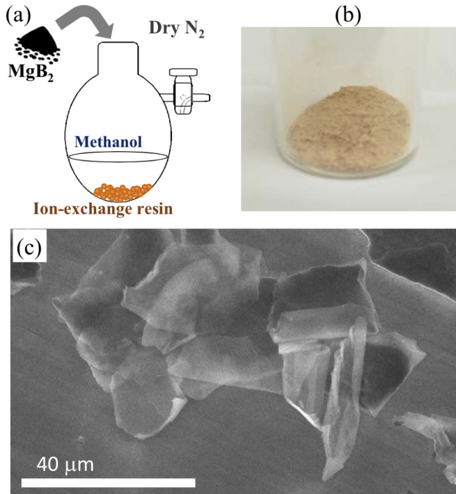
FIG. 1. (a) Schematic of the preparation procedure, (b) photograph of the sample powder, and (c) scanning electron microscope image of the free-standing hydrogen boride (HB) samples.
