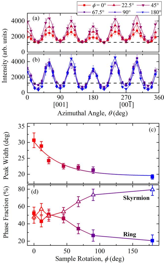
FIG. 2. Annular averages for (a)  $\phi = 0^\circ$ – $45^\circ$  and (b)  $\phi = 67.5^\circ$ – $180^\circ$ . (c) The azimuthal width of the six peaks of the skyrmion phase and (d) phase fractions from the skyrmion phase and ring phase, determined from their fractional contributions to the scattering intensity.
