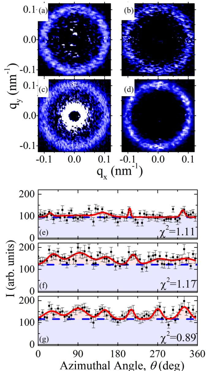
FIG. 5. SANS patterns from powdered  $\text{Cu}_2\text{OSeO}_3$  taken at (a)  $\phi = 0^\circ$ , (b)  $360^\circ$ , (c)  $720^\circ$ , and (d)  $1440^\circ$ . Azimuthal projections of the (e)  $\phi = 0^\circ$ , (f)  $720^\circ$ , and (g)  $1440^\circ$ , obtained at  $q = 0.11 \pm 0.035 \text{ nm}^{-1}$ .
