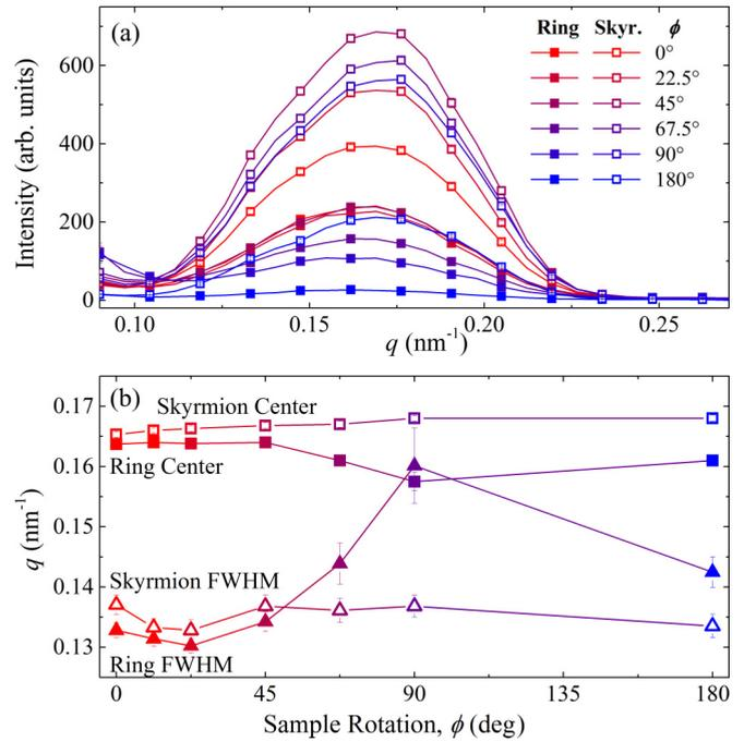
FIG. 3. (a) Summations of radial sector averages from Figs. 1(b) and 1(d)–1(g), taken at increments of  $60^\circ$  with  $\Delta\theta = \pm 3.5^\circ$  starting at  $0^\circ$  and  $30^\circ$ , capturing the radial distribution of the ring and skyrmion phases, respectively. Half of the data symbols are not shown for clarity. (b) Peak center and width for the sector averages of the ring and skyrmion features as a function of the sample rotation angle.
