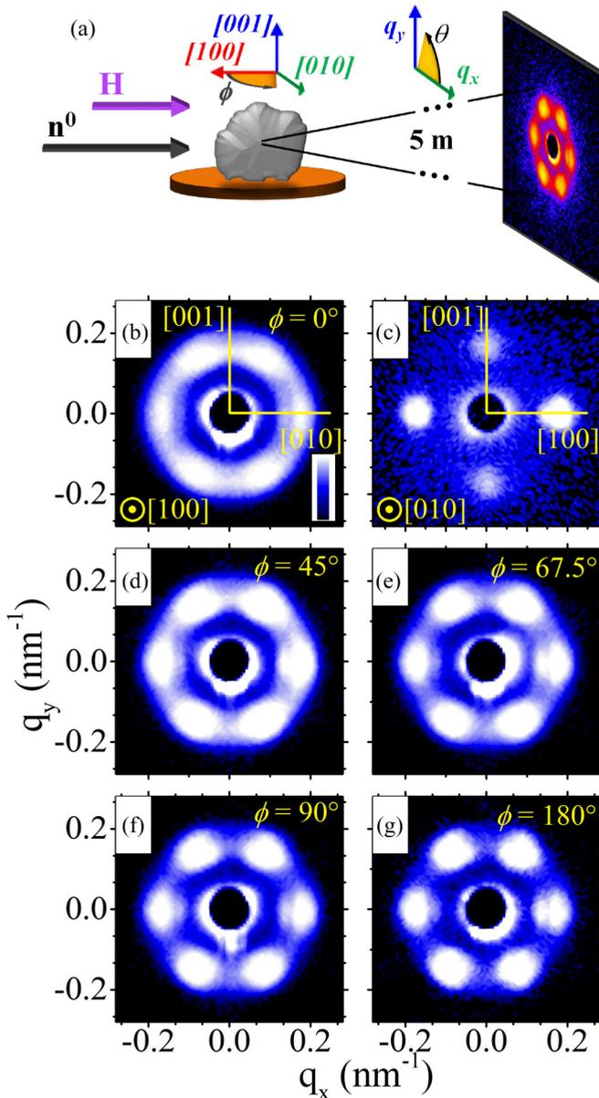
FIG. 1. (a) Diagram of SANS measurement setup. SANS patterns for (Fe, Co)Si initially aligned with the  $H \parallel [100]$  axis measured (b) with  $n^0 \parallel [100]$  and (c)  $n^0 \parallel [010]$ . SANS patterns with  $H \parallel n^0$  rotating the sample in the (001) plane by  $\phi =$  (d)  $45^\circ$ , (e)  $67.5^\circ$ , (f)  $90^\circ$ , then (g) back to the initial orientation ( $\phi = 180^\circ$ ).
