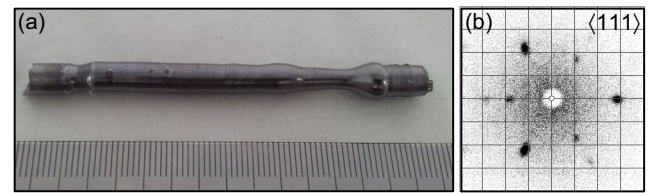
FIG. 2. Key characteristics of the single crystal grown for this study. (a) Optically float-zoned single crystal of \text{CuMnSb} . The scale on the bottom is given in millimeters. Growth direction was from right to left. (b) Threefold x-ray Laue pattern of a cubic \langle 111 \rangle axis.
