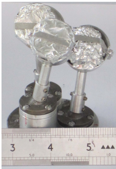
FIG. 1. The 192 g crystal of \text{PbMg}_{1/3}\text{Nb}_{2/3}\text{O}_3 used in the neutron scattering experiments, co-aligned and wrapped in aluminum foil.
