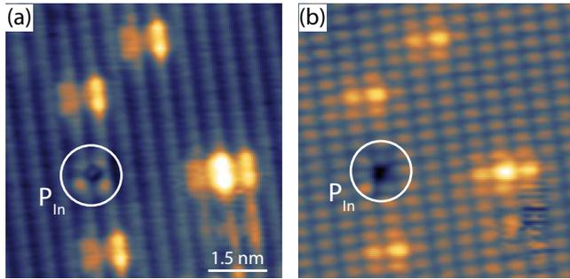
FIG. 6. High-resolution filled (a) and empty (b) states X-STM images of a  $P_{\text{In}}$  antisite in the surface, which is marked with a white circle. The images are acquired from the same spot of QW 2 in sample B at  $V_{\text{bias}} = -1.9$  V and  $V_{\text{bias}} = 1.5$  V with the same  $I_T = 30$  pA. The color ranges in both images are adjusted independently.
