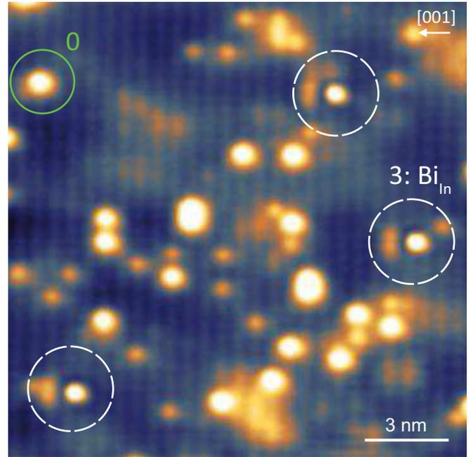
FIG. 7. High-resolution filled state X-STM image with potential  $\text{Bi}_{\text{In}}$  antisites [class (3)] with a valence of 5 in the surface layer next to commonly observed isovalent  $\text{Bi}_{\text{P}}$  substitutional atoms. An isovalent  $\text{Bi}_{\text{P}}$  atom in the cleavage plane [class (0)] is marked for comparison. The image is taken on F2 in sample B at  $I_T = 40$  pA and  $V_{\text{bias}} = -2.5$  V. The growth direction is indicated by an arrow.
