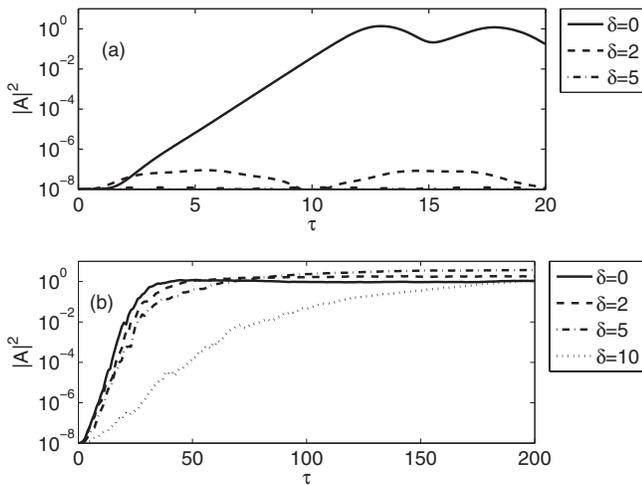
FIG. 3. Evolution of the scaled cavity mode intensity  $|A|^2$  (averaged over 100 runs) due to scattering of a (a) coherent pump ( $\Gamma = 0$ ) and (b) partially coherent pump ( $\Gamma = 5$ ) by a cold gas ( $\sigma = 0$ ) for different values of the pump-probe detuning  $\delta$ .
