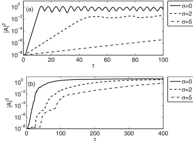
FIG. 4. Evolution of scaled cavity mode intensity (averaged over 100 runs) due to scattering of (a) a coherent pump ( $\Gamma = 0$ ) and (b) a partially coherent pump ( $\Gamma = 5$ ) showing the effect of increasing temperature (velocity spread,  $\sigma$ ). Note that in (a) the value of  $\delta$  used was  $\delta = \sigma$ , as this is the condition for maximum growth rate [11], whereas in (b) a value of  $\delta = 5$  was used.
