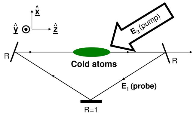
FIG. 1 (color online). Schematic diagram showing collective light scattering in a high-finesse unidirectional cavity. The misalignment of the pump field from the  $z$  axis is exaggerated.
