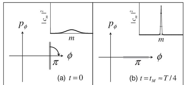
FIG. 2. Schematic picture of the probability distribution in phase space  $(\phi, p_\phi)$  for (a) the initial CSS and (b) the SSS at  $t = T/4$ . The insets: the corresponding distribution  $|c_m|^2$  as a function of  $m$  (or  $p_\phi$ ) obtained numerically with the parameters used in Fig. 1.
