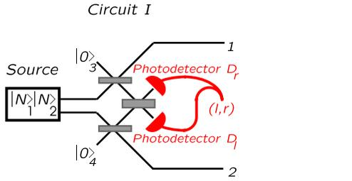
FIG. 1 (color online). Circuit I. Beam splitters couple some fraction  $f$  of the population from the principal modes 1 and 2 into ancillae modes 3 and 4, initially the vacuum. The ancillae are combined at a 50:50 beam splitter, and subjected to number-resolving photodetection.
