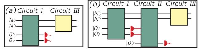
FIG. 2 (color online). (a) and (b) illustrate complete  $N00N$ -state generators in outline. Circuit I produces macroscopic superposition states nondeterministically. Circuit III consists of a  $\pi/2$  phase shifter and a 50:50 beam splitter, and performs final conversion to a  $N00N$  state. In (b) the Circuit I detection outcomes are feed-forward to Circuit II, which implements a correction step using a beam splitter of variable transmittance and an ancillary mode.
