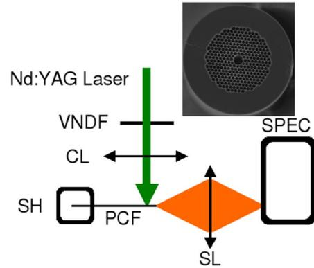
FIG. 1 (color online). Side view of the experimental setup. Variable neutral density filter (VNDF); 50 mm focal length cylindrical lens (CL); Sample holder (SH); 50 mm focal length spherical lens (SL); Spectrometer (SPEC). Inset: Scanning electron microscopy of the photonic crystal fiber used in the experiment (provided by Crystal Fibre A/S).
